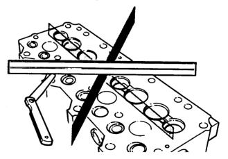
Fig.4 Checking cylinder head distortion.
