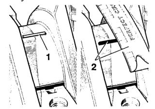
Fig.23 Using Plastigage to measure bearing clearance.
