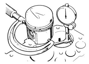
Fig.12 Measuring piston and bore diameters.
