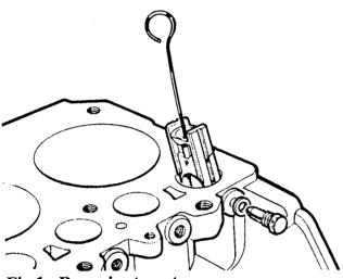
Fig.1 Removing tappets
