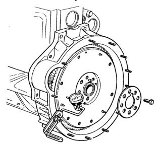
Fig.4 Measuring flywheel run-out
