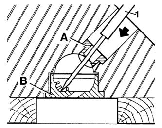
Fig.5 Removing hot plug A. Shroud B. Hot plug 1. Soft metal drift 11. To remove a hot plug, support the cylinder head face downwards on two pieces of timber, insert a thin soft metal drift through the injector shroud throat and tap the hot plug from the inside. Once removed in this way the hot plug must not be re-used.
