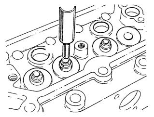
Fig.11 Fitting valve guide.
