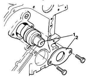
Fig.3 Removing camshaft 1 Camshaft
