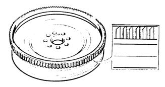
Fig.3 Fitting starter ring gear. (Inset shows squared edge of teeth downwards)
