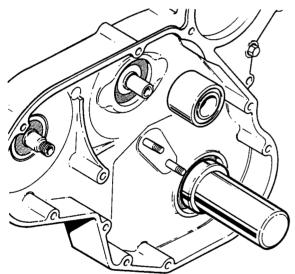
Fig.6 Fitting crankshaft seal with 18G 1456
