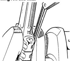
Fig.18 Measuring connecting rod end-float.
