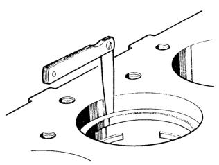
Fig.13 Measuring piston clearance.
