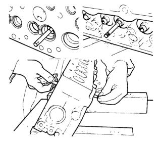
Fig.13 Fitting valve guide pilot.
