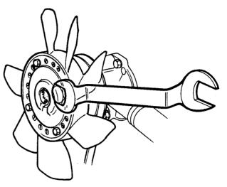
Fig.1 Using tool MS 1517 to release fan assembly
