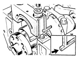
Fig.27 Fitting rear main bearing cap (inset shows chamfer on the cork seal).
