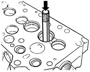
Fig.10 Removing valve guide.
