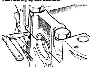
Fig.22 Checking main bearing cap nip.
