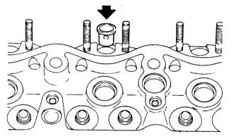
Fig 7 Fitting shroud
