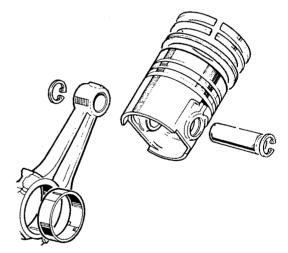
Fig.11 Connecting rod and piston.
