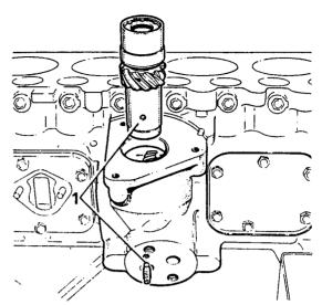
Fig.2 Removing skew gear 1 Grub screw and location
