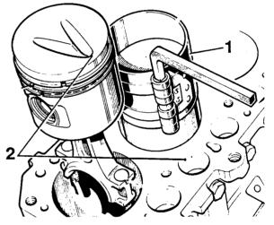
Fig.29 Fitting piston and connecting rod assembly. 1 Tool MS 38U3
