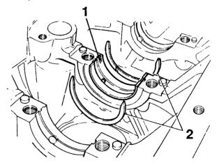
Fig.24 Crankshaft thrust washers. 1 Centre main bearing 2 Thrust washers
