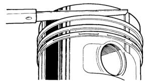
Fig.15 Measuring piston ring side clearance.
