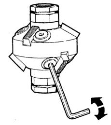
Fig.14 Valve seat cutter MS 621.
