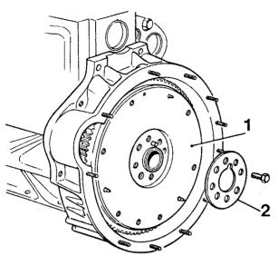
Fig.1 Flywheel location 1 Flywheel 2 Reinforcing plate
