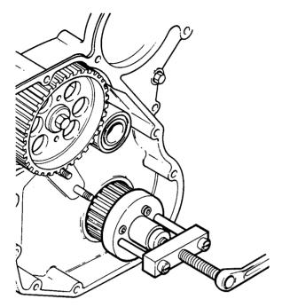
Fig.3 Crankshaft pulley removal with 18G 1464
