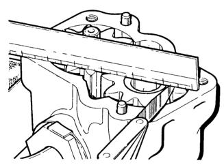
Fig.8 Measuring gear end float.
