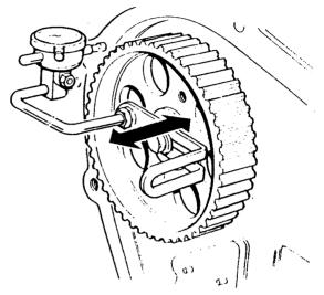
Fig.32 Measuring camshaft end-float.
