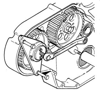
Fig.4 Injection pump pulley removal with 18G 1457
