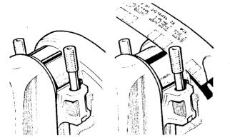
Fig.17 Using Plastigage to measure bearing clearance 1 Plastigage strip 2 Measuring flattened Plastigage
