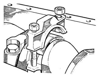
Fig.10 Connecting rod cap and bearing.
