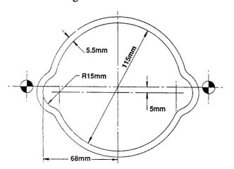
Fig.6 Sealant application - flywheel housing
