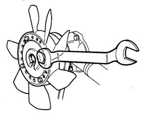
Fig.4 Using tool MS1517 to release the fan assembly
