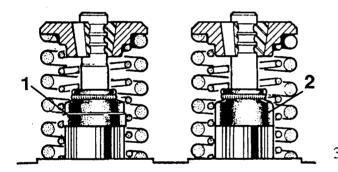
Fig.17 Valve seals 1.Exhaust valve seal 2.Inlet valve seal.
