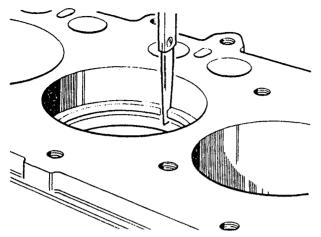
Fig.14 Measuring piston ring gap in bore.
