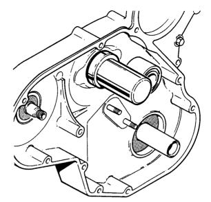
Fig.7 Fitting camshaft seal with 18G 1482
