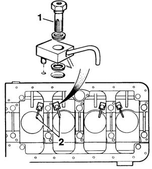
Fig.21 Jet adaptor locations 1 Adaptor retaining 'bolt' 2 Jet adaptors
