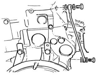
Fig.24 Cylinder head oil feed pipe.
