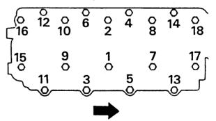
Fig.23 Cylinder head tightening sequence.
