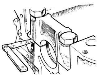
Fig.20 Checking main bearing caps for distortion.
