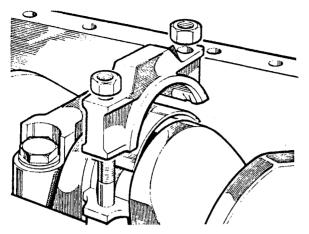
Fig.30 Fitting connecting rod cap.
