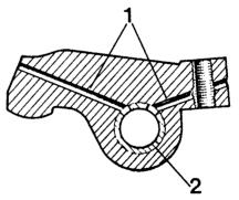
Fig.21 Cross section through rocker 1.Oil holes 2.Rocker shaft bush
