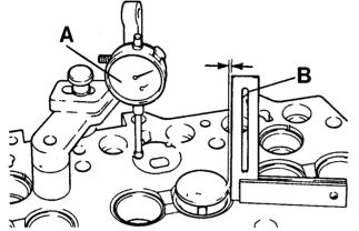
Fig.8 A. Checking stand-proud of hot plug. B. Checking valve guide wear.
