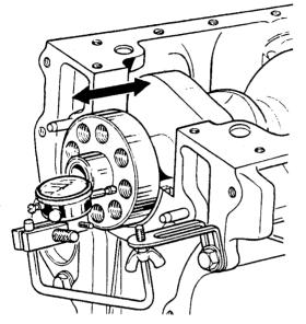
Fig.25 Measuring crankshaft end float.
