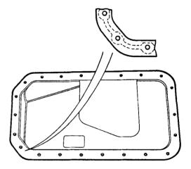
Fig.34 Applying sealant to sump.
