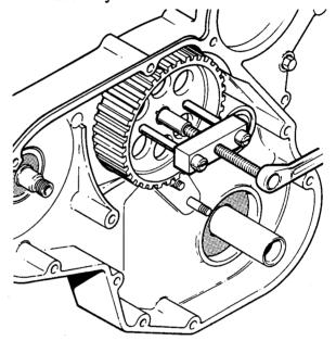
Fig.5 Camshaft pulley removal with 18G 1464
