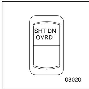
On vehicles with an engine shutdown, you will have to hold the manual throw switch in the UP position until normal engine pressures are reached. If you have one of these systems, a label on the control panel will say so.
