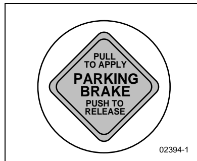
Full Truck Parking Brake Control Knob
