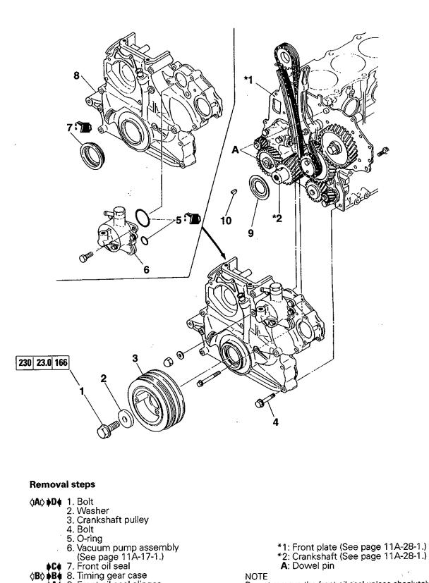
Do not remove the front oil seal unless absolutely necessary.
