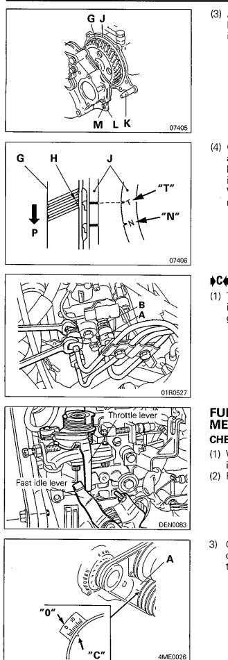
(3) Align the guide bar K of the flange plate J with the guide hole M of the front plate L and insert the front plate just before the injection pump gear G meshes with the idler gear.
