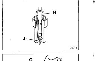
(e) Remove carbon deposited in the nozzle hole area of the nozzle tip 14 by turning the special tool Needle Cleaner
