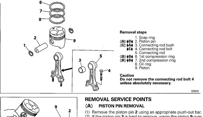
(2) If the piston pin **2** is hard to remove, warm the piston **9** over a heater or in hot water before removal.
