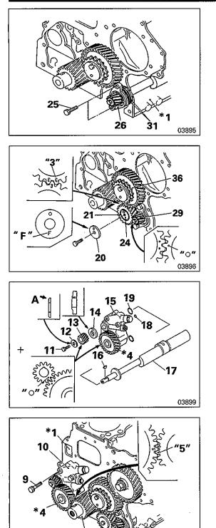
(b) Insert the completed balance shaft LH assembly 16 into the crankcase assembly \*1, set it in position with the dowel pin on the crankcase assembly and secure it with bolts 25.
