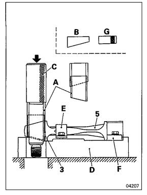
(2) Use the special tool to replace the connecting rod bush 3. Component Parts of Special Tool MH062455 – Connecting Rod Bush Puller Kit
