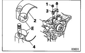
B4 PISTON AND CONNECTING ROD ASSEMBLY INSTALLATION
