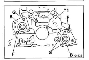
(4) Secure the plate **B** to the crankcase **\*1** using bolt **F** [M8x1.25 mm (0.042 in.)]
