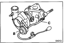
(2) Using a tester, apply pressure to the actuator **B** and read the pressure at which the rod **C** begins to move [approximately 1 mm (0.04 in.)].
