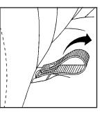
2. Pull the seat loop located where the seatback and seat cushion meet. The seat cushion will release and allow you to tilt it toward the front of the vehicle.
