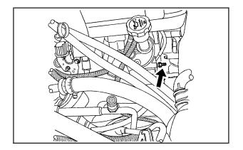
The remote negative (-) terminal is a stud located on the right front of the engine, where the negative battery cable attaches.
