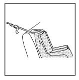
If the position you are using does not have a headrest or head restraint and you are using a single tether, route the tether over the seatback.
