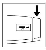
Pressing this button at the end of the shift lever turns on and off the tow/haul mode.
