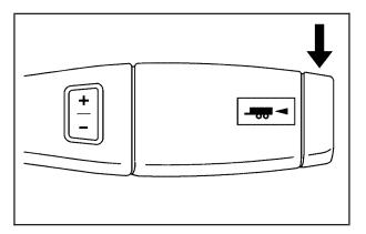
The vehicle has a tow/haul mode. The tow/haul mode adjusts the transmission shift pattern to reduce shift cycling, providing increased performance, vehicle control, and transmission cooling while towing or hauling heavy loads.
