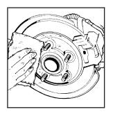
7. Remove any rust or dirt from the wheel bolts, mounting surfaces, and spare wheel. 8. Install the spare tire.
