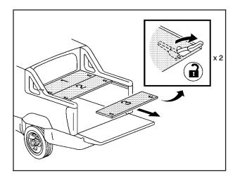
2. Unlock the cargo panel 3 by pulling forward on the driver side and passenger side cargo panel latches, located on the bottom of each cargo panel.
