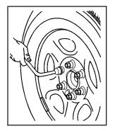
Use the wheel wrench to loosen all the wheel nuts. Turn the wheel wrench counterclockwise to loosen the wheel nuts. Do not remove the wheel nuts yet.
