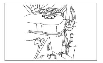
The coolant surge tank is located in the engine compartment on the passenger side of the vehicle. See *Engine Compartment Overview on page 5-14* for more information on location.
