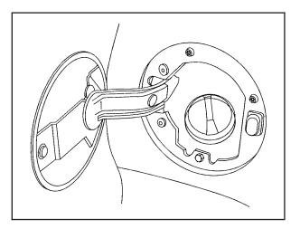
The tethered fuel cap is located behind a hinged fuel door on the driver side of the vehicle. If the vehicle has E85 fuel capability, the fuel cap will be yellow and state that E85 or gasoline can be used. See *Fuel E85* (85% Ethanol) on page 5-8.
