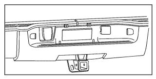
Your vehicle is equipped with the seven-wire trailer towing harness. This harness with a seven-pin universal heavy-duty trailer connector is attached to the rear bumper beam. It is located next to the integrated trailer hitch. The seven-wire harness contains the following trailer circuits:
