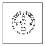
When the engine is not running, but the ignition is on, this gage shows the battery's state of charge in DC volts.
