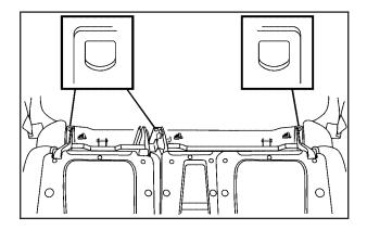
The top tether anchors are located on the back of the rear seat frame above the floor for each rear seating position. Fold down the rear seatback(s) to access the anchors. See *Rear Seat Operation on page 1-13*. Be sure to use an anchor located on the same side of the vehicle as the seating position where the child restraint will be placed.
