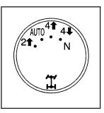
The transfer case knob is located to the left of the instrument panel cluster.
