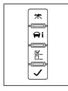
The buttons are the trip/fuel, vehicle information, customization, and set/reset buttons. The button functions are detailed in the following pages.
