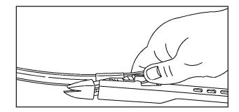
3. Install the new blade onto the arm connector and make sure the grooved areas are fully set in the locked position.
