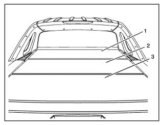
The panels are embossed on the upper center portion with the numbers 1, 2 and 3. There are also numbered labels on the bottom of the panels. The numbers on the top and bottom of the panels will be used as reference when removing, storing and reinstalling the panels.
