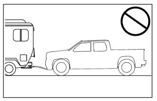
*Notice:* If the vehicle is towed with all four wheels on the ground, the drivetrain components could be damaged. The repairs would not be covered by the vehicle warranty. Do not tow the vehicle with all four wheels on the ground.
