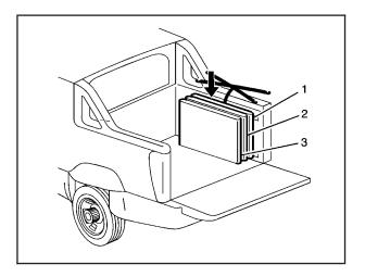
2. Starting with cargo panel 1, load the cargo panel with the latches facing up toward the side of the cargo box.
