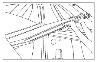
1. Starting with cargo panel 1, place the latches in the unlocked position. Place cargo panel 1 on the cargo area rails while holding the back of the cargo panel up.
