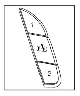
The controls for this feature are located on the driver's door panel, and are used to program and recall memory settings for the driver's seat, outside mirrors, and the adjustable throttle and brake pedal. To save seating positions in memory:
