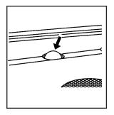
The solar sensor, located in the defrost grille, middle of the instrument panel, monitors the solar heat. Do not cover the solar sensor or the system will not work properly.
