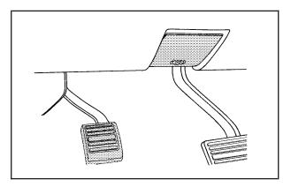
For vehicles with a release handle, set the parking brake by holding the regular brake pedal down, then pushing down the parking brake pedal. If the ignition is on, the brake system warning light will come on. See *Brake System Warning Light on page 3-36.*
