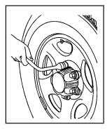
If the vehicle has a center cap, place the chiseled end of the wheel wrench in the slot on the wheel and gently pry the cap out.
