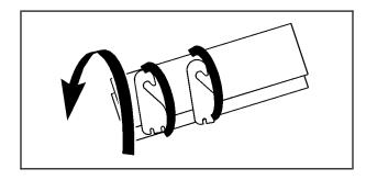
4. Take the storage strap and wrap it around the package. Finally, attach the hooks to the webbing and place the straps inside the top box storage compartment.
