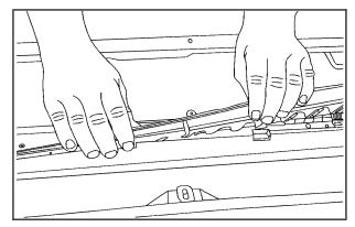
2. Pull up on the rear side of the drain grate, tilt it toward the front of the vehicle, and pull it out.
