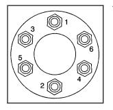
Tighten the nuts firmly in a crisscross sequence as shown by turning the wheel wrench clockwise. When you reinstall the full-size wheel and tire, you must also reinstall the either the center cap or the bolt-on hub cap, depending on what your vehicle has.
