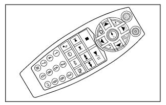
$\overset{(}{\cup}$  (Power): Press this button to turn the video screen on and off.
