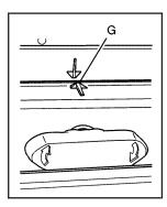
Be sure to align the rear glass side-to-side using the alignment arrows (G).
