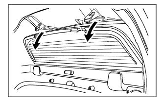
4. With the rear glass tilted at an angle, place the bottom edge in the lower channel of the window frame.
