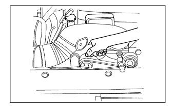
4. With the coolant surge tank pressure cap off, start the engine and let it run until you can feel the upper radiator hose getting hot. Watch out for the engine cooling fan.
