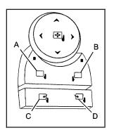
Vehicles with outside power foldaway mirrors have controls located on the driver door armrest.
