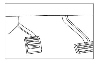
For vehicles without a release handle, set the parking brake by holding the regular brake pedal down, then pushing down the parking brake pedal. If the ignition is on, the brake system warning light will come on. See *Brake System Warning Light on page 3-36.*
