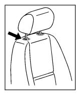
Pull the head restraint up to raise it. To lower the head restraint, press the button, located on the top of the seatback, and push the restraint down.
