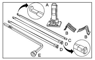
The tools needed are the jack (A), the wheel blocks (B), the jack handle (C), the jack handle extensions (D), and the wheel wrench (E).
