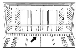
The removable Midgate drain grate is located near the base of the Midgate.
