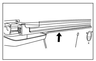
1. Line up the clips on the vehicle with the slots in the grate and firmly push the grate down.
