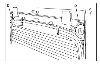
Turn both glass lock knobs (D), located at both top corners of the storage pocket, to the locked position. Push in on the corner of the rear glass to allow the lock knob to engage more easily.
