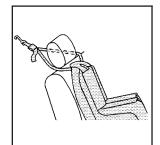
If the position you are using has an adjustable headrest or head restraint and you are using a dual tether, route the tether around the headrest or head restraint.
