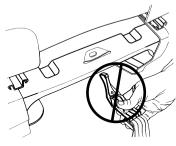
If the tether strap is clipped incorrectly (as shown) the child safety seat may not be retained properly in the event of a collision.
