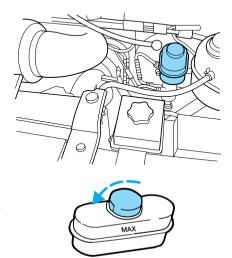
4. Use only a DOT 3 brake fluid certified to meet Ford specifications. Refer to Lubricant specifications in the Capacities and specifications chapter.
