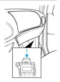
For commercial stripped chassis vehicles, the fuel pump shut-off switch is located on a bracket above the brake pedal.
