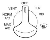
The air conditioning compressor will operate in all modes except VENT and FLR. However, the air conditioning will only function if the outside temperature is about  $10^{\circ}\text{C}$  ( $50^{\circ}\text{F}$ ) or higher.
