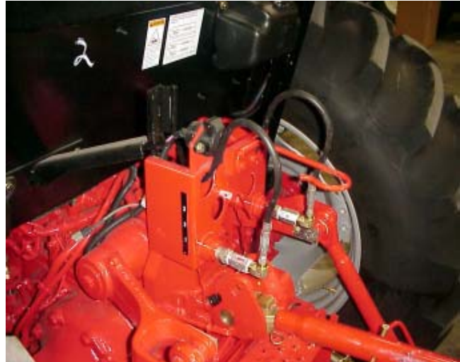
Tractor Hydraulic Used for Cylinder
