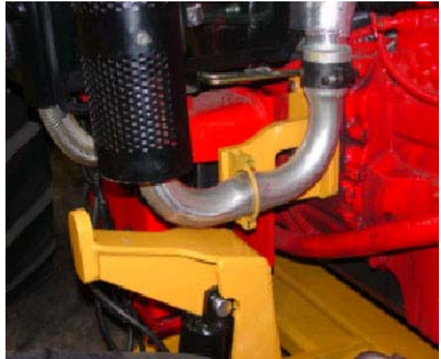
Replacement Exhaust Pipe Installed
