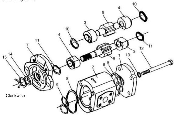
Fig. 7-1 clockwise gear pump
