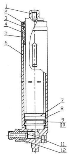
Fig.8-5 Lifting cylinder (Used in fig.10-1, 10-4)
