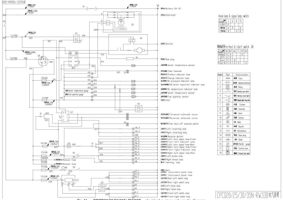
Fig.11 CPCD20/25/30/35N-RW33B electrical system schematic diagram
