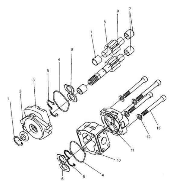
Fig. 7-3CBHZG clockwise (Right) rotation gear pump
