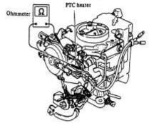
Ensure PTC heater becomes hot when engine is started.(Simple check method)
