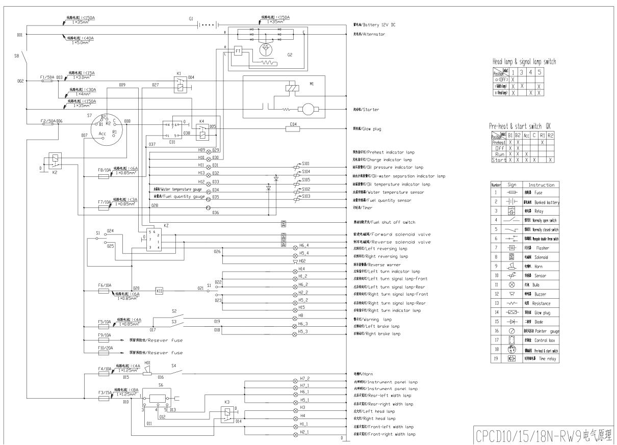
Fig.2 CPCD10/15/18N-R W9/W10 electrical system schematic diagram
