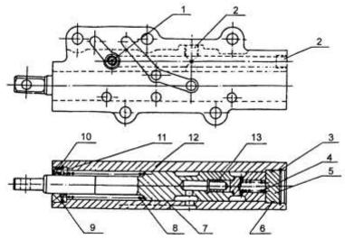
1 threaded plug 5plug6 o-ring 2 threaded plug7 inching valve lever
