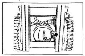
5) Support mast assembly with wire ropes.
