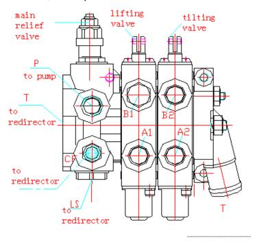
Fig.7-4 Control valve for 1t ∼ 3.5t forklift truck
