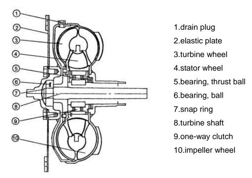
Fig.2-4 Torque converter
