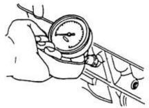
6). Cylinder compression in cylinders should not be less than 80% of the highest reading.
