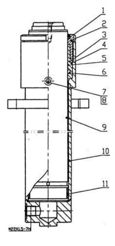
Fig. 8-8 free lifting cylinder (used in 8-2, 8-3)
