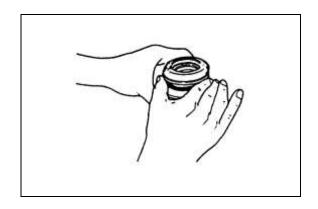
8) Remove O-ring and Y-ring in the inner hole of guiding bush (see Fig. disassembly and installation of lifting iack).
