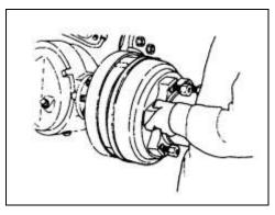
adjusting nut adjusting hole plug brake dust cover
