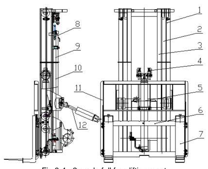
Fig.8-4 3 grade full free lifting mast
