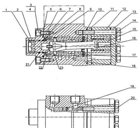
Fig. 5-2 cycloidal rotor full hydrostatic power steering gear
