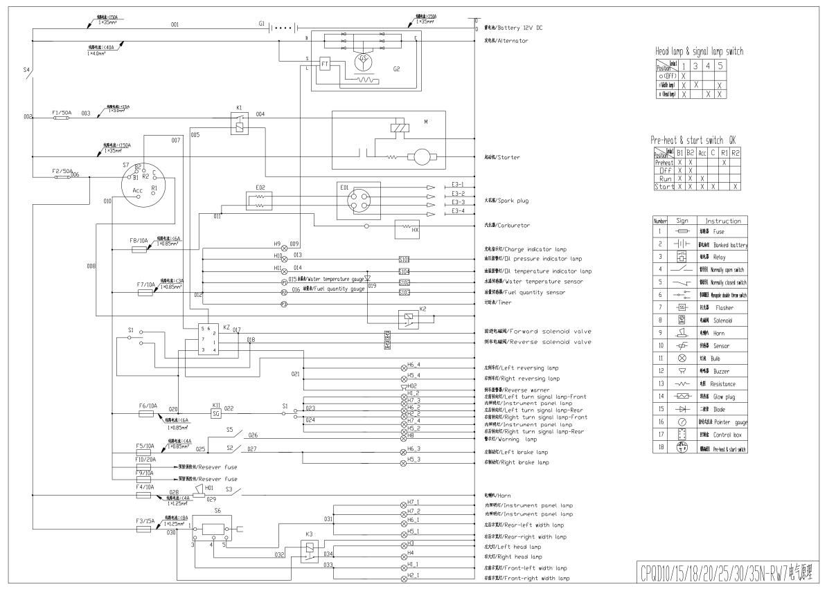
Fig.1 CPQD10/15/18/20/25/30N-RW7 electrical system schematic diagram
