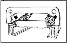
2) Slide inner mast, then remove lifting cylinders.
