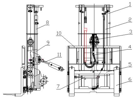
Fig.8-3 Containers forklift mast
