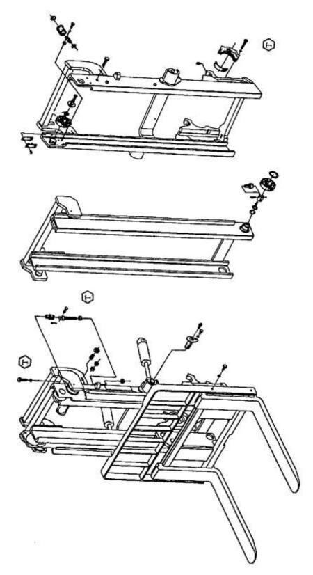
N30M300-000000-000 Lifting Mast assembly
