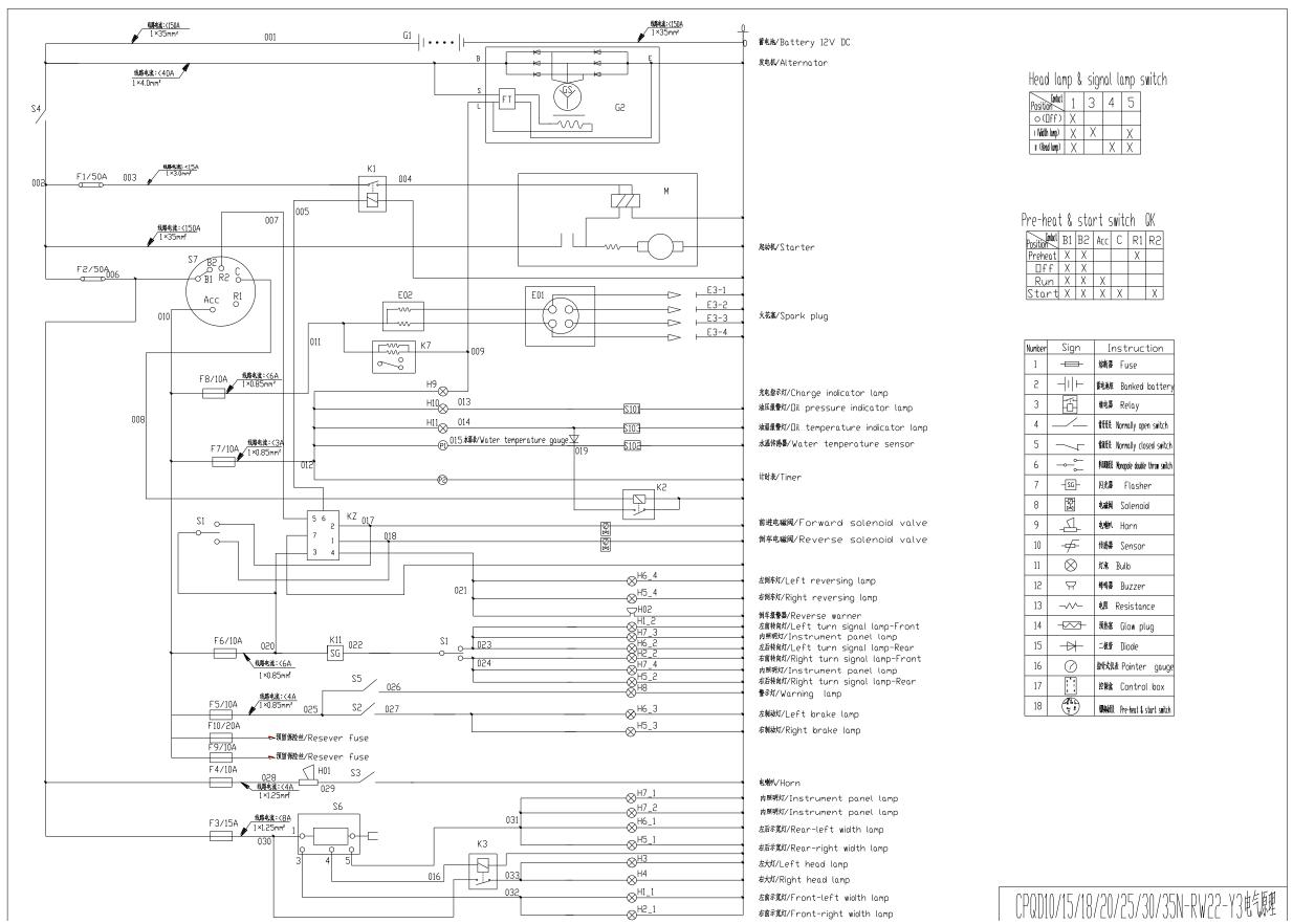
Fig.6 CPQD10/15/18N-RW21-Y3、CPQD20/25/30/35N-RW22-Y3 electrical system schematic diagram
