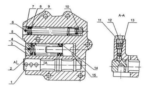
**Main pressure valve:** also called fixed pressure valve, the oil pressure for controlling the hydrodynamic clutch is at 1.1MPa ~1.4MPa, assigns the oil to the relief valve, then to torque converter.
