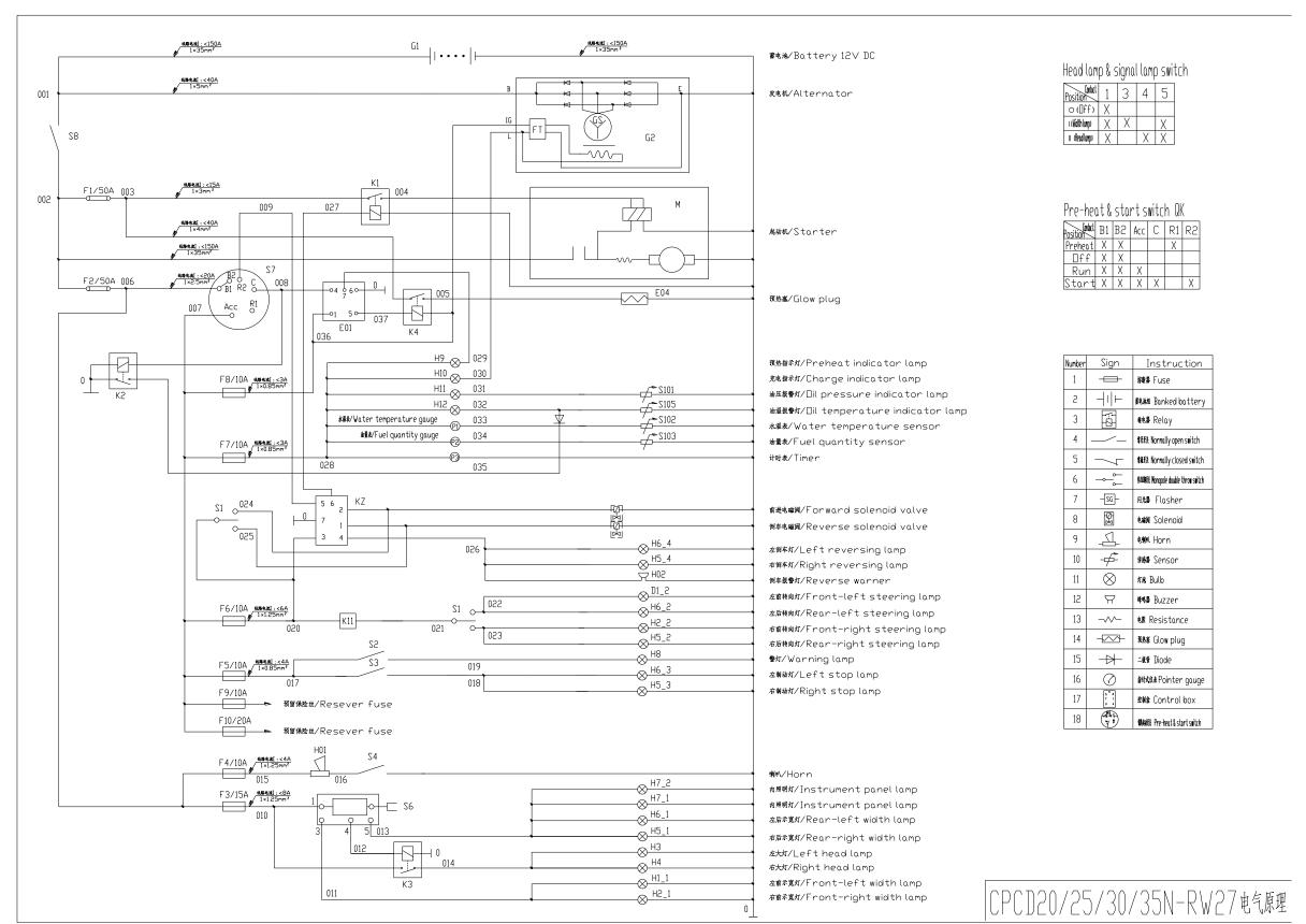
Fig.8 CPCD20/25/30/35N-RW27 electrical system schematic diagram
