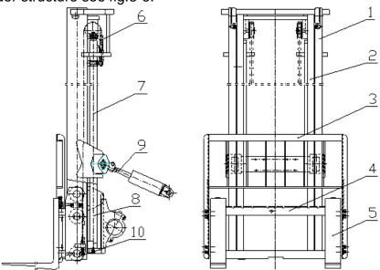
Fig. 8-1 Double stage wide view mast
