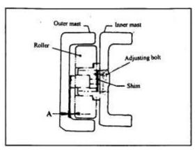
b. Dimension:0mm  $\sim$  0.5mm (2.5t  $\sim$  3 t).One or two may not using rubber pad; Dimension:0.1  $\sim$  0.6mm if no rubber pad.
