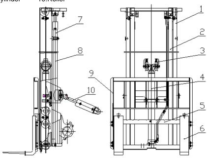
Fig.8-2 Double grade full free lifting mast
