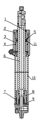
Fig.8-7 Lifting cylinder (left) (used in fig.8-2, 8-3)
