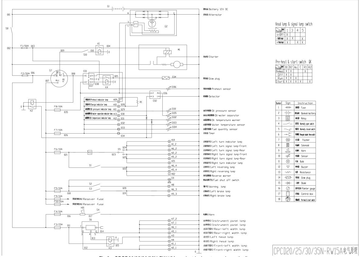
Fig.3 CPCD20/25/30/35N-RW15A electrical system schematic diagram
