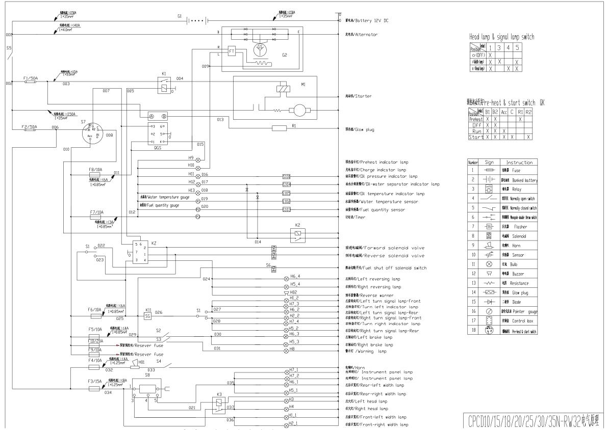
Fig.9 CPCD10/15/18/20/25/30/35N-RW32 electrical system schematic diagram
