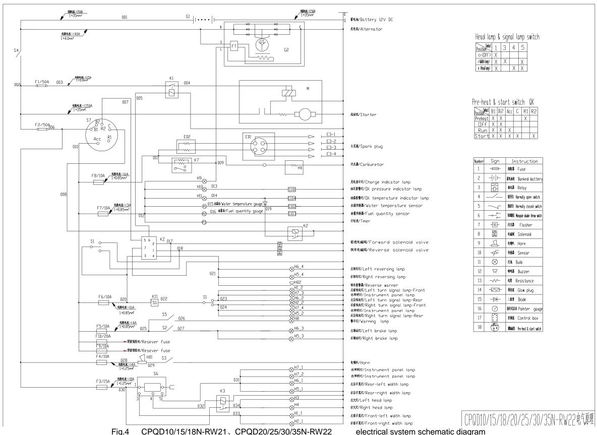
CPQD10/15/18N-RW21、CPQD20/25/30/35N-RW22 electrical system schematic diagram
