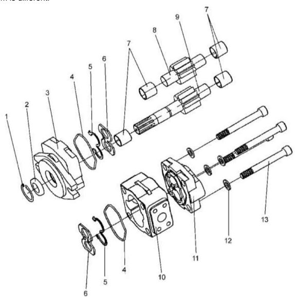
Fig. 7-2CBHZG counterclockWise rotation gear pump (left)
