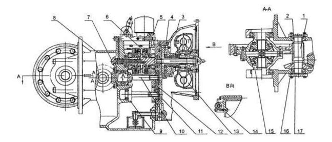
1 Shaft, Final Pinion 2 tapered roller bearing 3.torque converter shell assy
