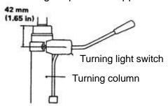
After installing turn signal lamp switch ,insure the distance between turn signal lamp switch and top of steering column is 42mm.
