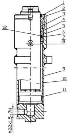
Fig. 8-10 free lifting cylinder (used in 8-2、8-3)
