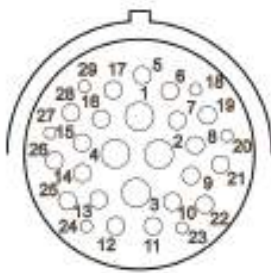
Fig. 10 Granite BodyLink III 29-pin Connector, Wire Insertion Side of Connector.
