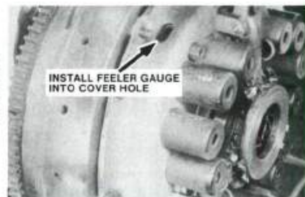
Fig. 165—On Borg and Beck continuous type clutch, insert feeler gauge through holes in clutch cover to check clearance between adjusting screws and pressure plate.
