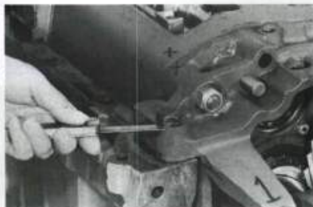
Fig. 176—Measure clearance between head of mounting bolts and transmission housing. Clearance is determined by thickness of shims installed beneath mounting bolt bushings.
