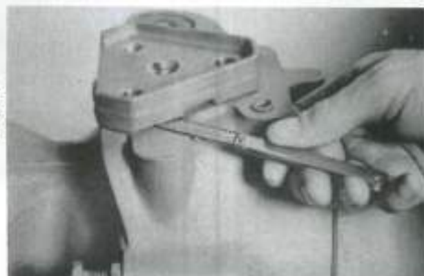
Fig. 33—To set swivel bearing preload, measure gap between swivel pin and swivel housing with a feeler gage. Refer to text.
