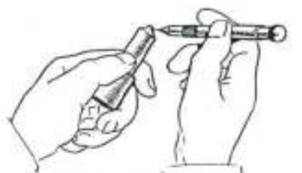
Fig. 122—Use a pin vise and proper size cleaning wire to probe all carbon from the four injection spray holes in each nozzle tip.
