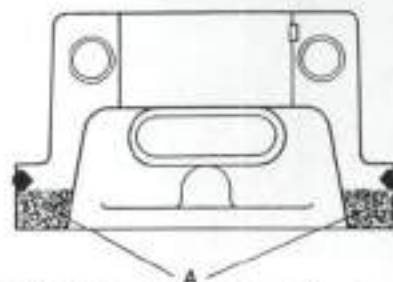
Fig. 93—When installing front main bearing cap on three-cylinder engines, apply light coat of RTV silicone sealer to mounting surface of cap indicated by shaded area "A".
