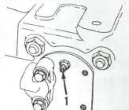
Fig. 240—On all models except 1594 and 1690, air bleed fitting (1) is located on rockshaft cylinder.
