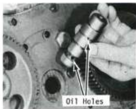
Fig. 86—When installing idler shaft, be sure oil holes are positioned downward toward the crankshaft.
