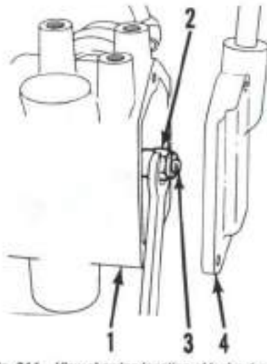
Fig. 244—View showing location of locknut used to adjust connecting link on cab or platform equipped models.
