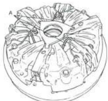
Fig. 168—Use retainers (A) made from stiff wire to hold pto clutch release levers down during removal and installation of clutch. Do not use soft wire or welding rod as they will not retain pressure of clutch springs.
