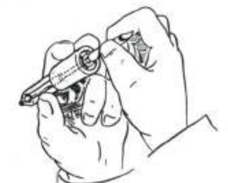
Fig. 120—Use a seat scraper to clean all carbon from needle seat in tip of nozzle by rotating scraper while pressing it against seat.
