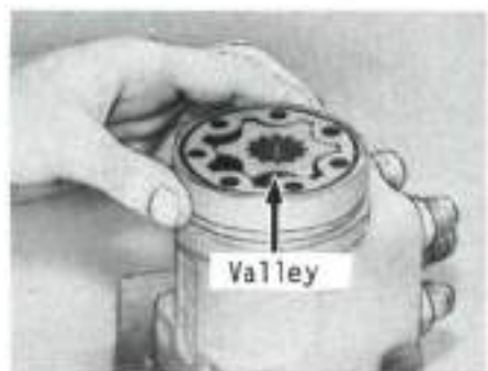
Fig. 59—Rotor is properly "timed" to valve spool by engaging drive shaft splines in such a way that one of the valleys in rotor is aligned with drive pin slot in drive shaft.
