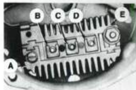
Fig. 138—Rectifier bridge has a grounded mounting screw "A" and an insulated screw "E" which is connected to output terminal. "B", "C" and "D" are individual diode leads.
