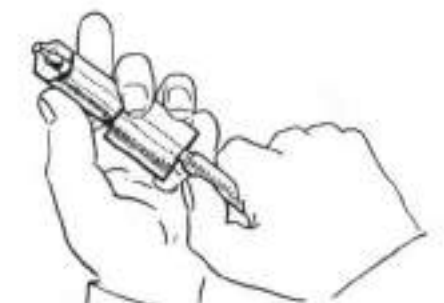
Fig. 121—Remove any carbon from dome (tip) cavity with dome cavity cleaner as shown.
