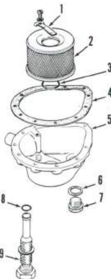
Fig. 237—Exploded view of hydraulic suction filter assembly used on Models 1494 and 1594. Models 1390, 1394, 1490 and 1690 are similar. Filter screen (9) is used on power shift models only.
