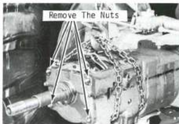
Fig. 195—Use a hoist and chain to support power shift unit as shown when removing and installing unit from range gearbox.
