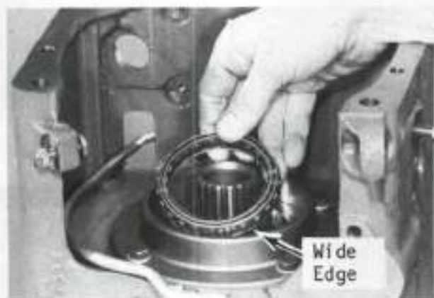
Fig. 204—Install spring clutch into carrier housing with wide edge facing inward as shown.
