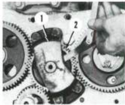
Fig. 88—Check clearance between idler gear (2) and support bracket (1) using a feeler gage. Add or remove bracket mounting shims to adjust clearance.
