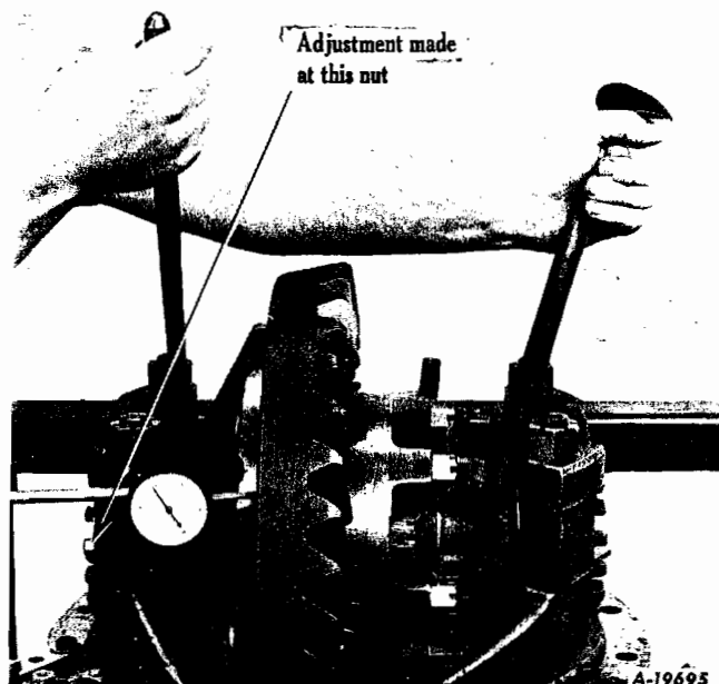
Fig. 9 - Adjusting differential bearing pre-load.
