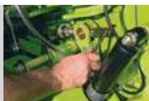
Mechanical shear bar adjustment
