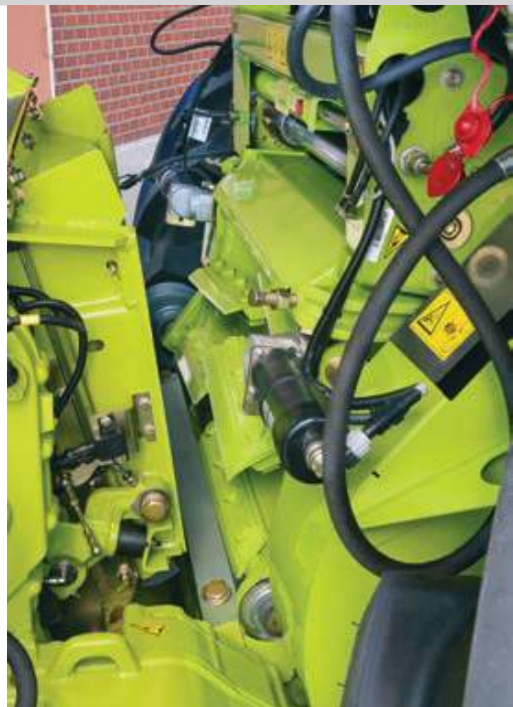
Ease of access to knife drum
