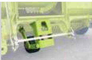
Support wheel for optimal ground-contour following
