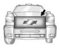
2. Slide the channels of the cover down the back edge of the grille on both sides.
