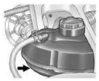
The coolant surge tank is located near the center of the engine compartment. See *Engine Compartment Overview on page 10-3* for location.
