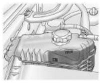
The coolant surge tank is located in the engine compartment on the passenger side of the vehicle. See *Engine Compartment Overview on page 10-3* for location.
