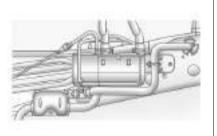
If the vehicle includes an FOH, it will enhance heater performance and will reduce the amount of time it takes to warm the inside of the vehicle in cold conditions below or equal to 4°C (39°F). The FOH is installed on the frame rail on the driver side of the vehicle and uses diesel fuel to heat the engine coolant, which warms up the passenger cabin air. The FOH will turn on if all of the following conditions exist:
