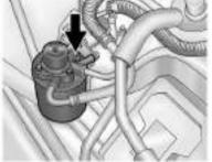
Open the fuel filter vent valve by 5. turning the screw counterclockwise several full turns. The vent valve is located on top of the fuel filter housing.
