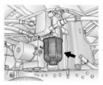
The fuel pump screen should be inspected and cleaned if necessary at each fuel filter inspection or replacement.
