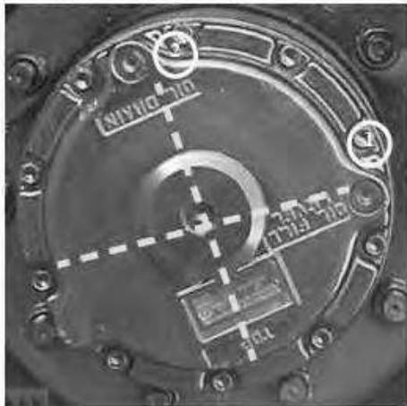
You need to dismantle the wheel to inspect it and change the oil. To do this, immobilise the machine and raise it with a jack, hoist or stabilising cylinder.
