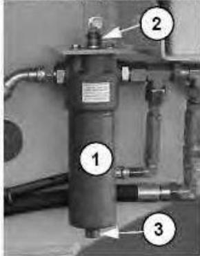
Photo 16 Travel circuit hydraulic oil filter
