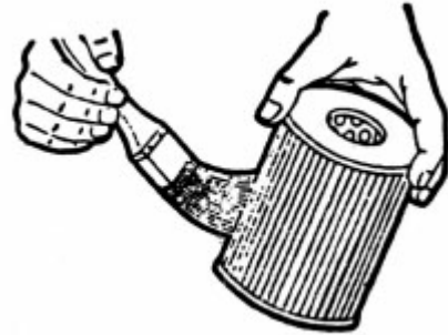
Fig.6-40 service and clean the filter core of air filter
