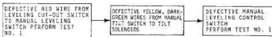
Fig. 7-Combine Will Level Automatically but Not Manually in Either Direction
