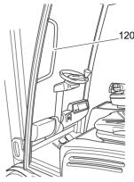
An additional step is provided for the driver position extension ( $\bigcirc$ ).
