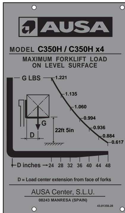
Load charts for C350H / C350H x4 front wide axle and and quick attach fork carriage (500 mm. load centre)
