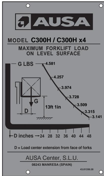
Load charts for C300H / C300H x4 front narrow axle and and quick attach fork carriage (500 mm. load centre)
