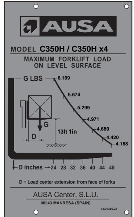
Load charts for C350H / C350H x4 front narrow axle and and quick attach fork carriage (500 mm. load centre)
