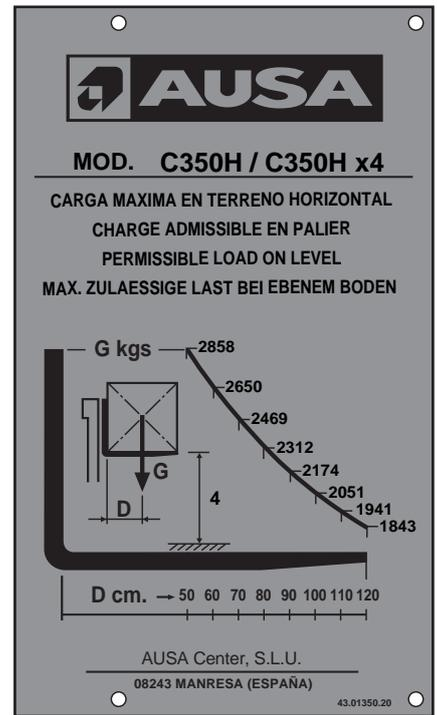
Load charts for C350H / C350H x4 front narrow axle and and quick attach fork carriage (600 mm. load centre)
