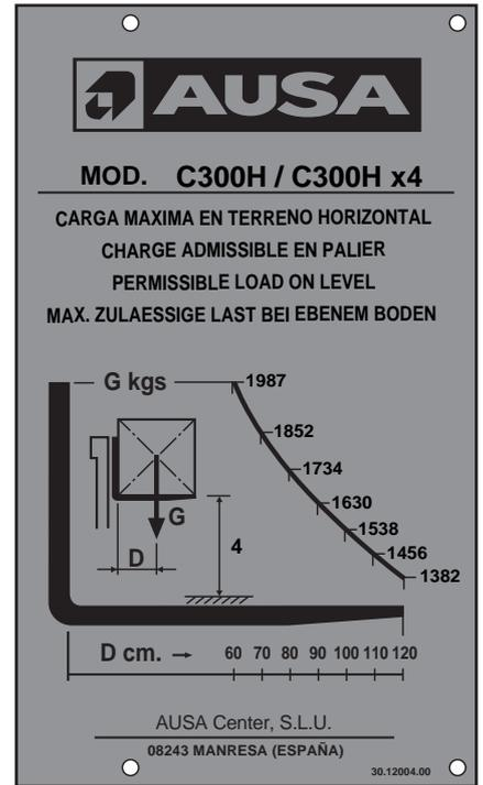
Load charts for C300H / C300H x4 front narrow axle and and quick attach fork carriage (600 mm. load centre)
