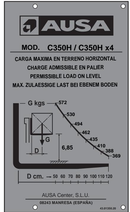
Load charts for C350H / C350H x4 front wide axle and and quick attach fork carriage (600 mm. load centre)
