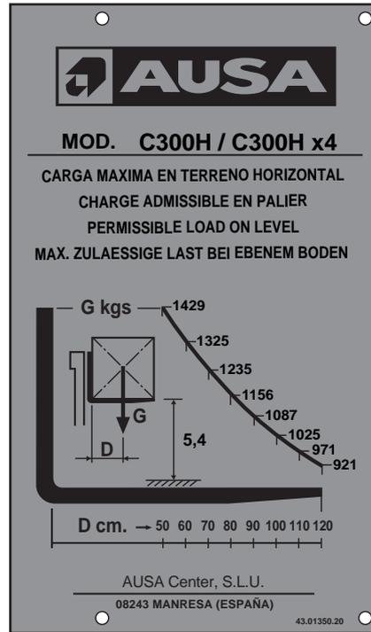
Load charts for C300H / C300H x4 wide front axle and quick attach fork carriage (600 mm. load centre)
