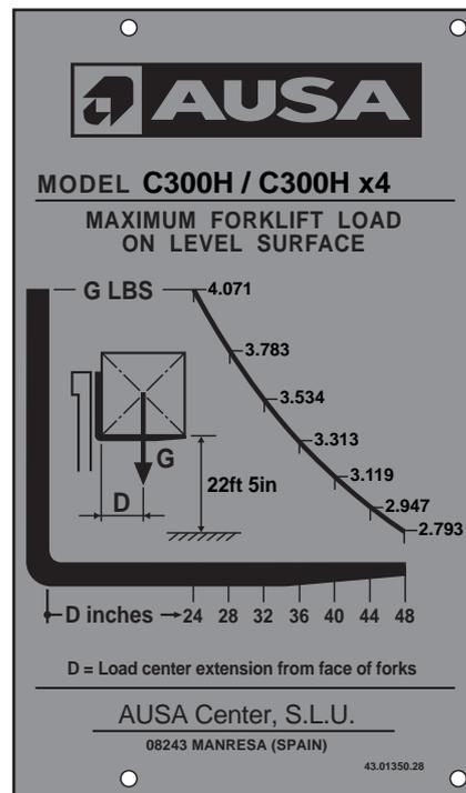
Load charts for C300H / C300H x4 wide front axle and quick attach fork carriage (500 mm. load centre)
