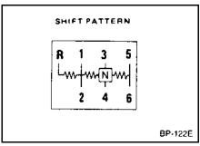
Familiarize yourself and others operating the vehicle with the manual transmission, the gear shift pattern and clutch operation. When using the clutch, be sure that the clutch is fully engaged or disengaged. Never operate the vehicle with the clutch partially engaged.
