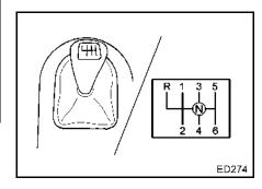
The transmission gear shift lever is located on the right of the driver's seat. When shifting gears, depress the clutch pedal fully and move the lever firmly. When the shift lever is moved into reverse, the backup lights come on and the backup buzzer sounds. The backup lights and buzzer are located on the rear of the vehicle
