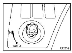
The engine throttle control knob, located to the left of the steering column, can be used to adjust engine idling speed. Normal engine idling speed is 550 rpm. If equipped with automatic transmission, make sure the engine idling speed is 550 rpm at the forward range.
