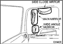
Check the outside mirrors daily for damage, position and visibility. Also check that the mirror mounting bolts are properly tightened.
