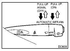
The hazard warning flasher switch is located on the lever mounted on the right side of the steering column.
