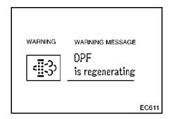
Wait approximately 25 minutes. (when it is operated after the engine has already warmed up.) When the DPF regenerating warning is no longer displayed on the multi-display monitor, regeneration is completed.
