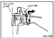
2.Pull the tilt lock lever out all the way. This releases the main hook which holds the cab body to the cab frame. The torsional springs will cause the cab to raise slightly.
