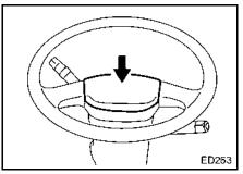
The horn pad is mounted in the center of the steering wheel. Press on the pad to sound the horn.
