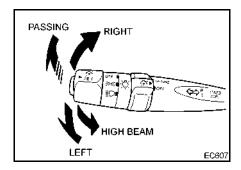
To operate the left turn signal, pull the turn lever on the left side of the steering column down beyond the resistance. To operate the right turn signal, push the lever up beyond the resistance. The lever will automatically return to the neutral position after the turn is completed. When operating the left or right signal, confirm that the TURN SIGNAL AND HAZARD indicator light flashes. When the ON-OFF intervals are unusually short, the bulb is probably burned out.
