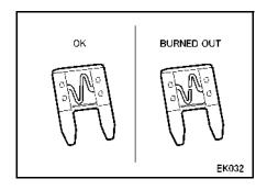
Install a new fuse with the same current rating as that specified for the circuit.
