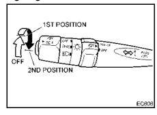
Turn the knob on the end of the switch lever to the 1st or 2nd position to operate the following lights.
