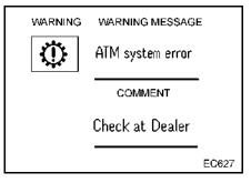
1.The automatic transmission system warnings will be displayed when the TCM detects a malfunction. At this time a diagnostic trouble code (DTC) is set in the TCM and transmission cannot be shifted. Depending on the malfunction, the TCM does not respond to gear shifting operation and the current gear is fixed.
