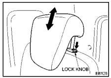
The height of the headrest can be adjusted manually. Adjust the headrest height while pressing the lock knob.
