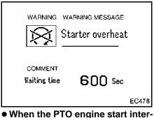
rupt warning is operated, a warning and a warning message will be displayed. These warnings indicate that the engine is unable to start because the PTO switch is in the ON position. If this occurs, turn the PTO switch to the OFF position, and then start the engine.
