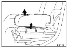
The front of the driver's seat can be raised by pulling up the lever at the left side of the seat base.
