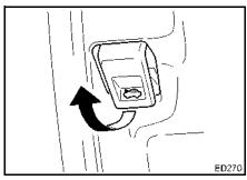
2. Disengage the front lid hook. Push up the front lid and secure it with the rod.
