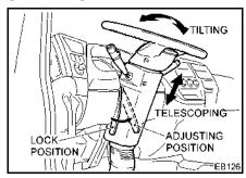
The steering wheel telescopes 2.95 inches (75 mm) and tilt angle 9.5°. Position the driver's seat before adjusting the steering wheel. Loosen the lock lever and adjust the steering wheel to the desired position. After adjustment, securely tighten the lock lever.
