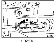
: Lubricate with a grease gun.
