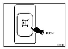
This switch located on the instrument panel to the left of the steering column, couples and uncouples power flow to the transmission PTO. To turn the PTO ON, idle the engine, depress the clutch pedal fully, and depress the switch. The PTO indicator and operation message will come on. To turn the PTO OFF, idle the engine, depress the clutch pedal fully, and depress the switch. The PTO indicator and operation message will go out.
