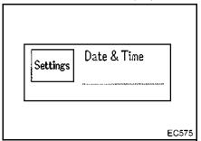
To set the calendar and clock display, press the mode select switch or the select switch for more than 1 second or turn the return switch for more than 1 second while the calendar and clock display is shown. A cursor will be displayed and blink on the year position.
