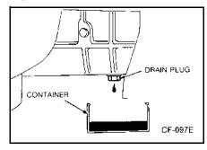
2. After draining, replace the gasket of the drain plug with a new one. Reinsert the plug and tighten the plug. Tightening torque: UD1800 thru UD3300 MLS63 72 to 89 ft·lbf (98 to 120 N·m) (10 to 12 kgf·m) UD2600 and UD3300 MLS63 72 to 94 ft·lbf (98 to 130 N·m) (10 to 13 kgf·m) MPS63 87 to 101 ft·lbf (118 to 137 N·m) (12 to 14 kgf·m)
