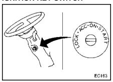
The ignition key switch, located on the right side of the steering column, has four positions:
