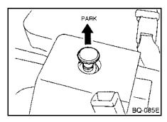
The parking brake valve is located to the rear of the gear shift lever. Pull the knob up to operate the parking brake. When the knob is pulled up, the PARKING BRAKE warning light comes on. To release the parking brake, press the knob down. The warning light will go out.
