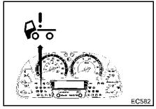
When the warning light comes on and the warning buzzer sounds, immediately move the vehicle to a safe place. To do this, apply the brake slowly.
