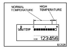
If the engine coolant temperature (ECT) significantly increases, an overheat warning with a 2-phase indication (amber: moderate, red: severe) will appear.
