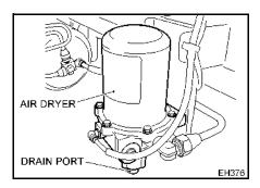
Visually check to be sure that water drains from the drain port of the air dryer. Water will drain when the air pressure governor stops pressurization. The governor stops pressurization when the air pressure in the reservoir reaches the upper level of the normal operating pressure range. When the sound of air supplied to the reservoir can no longer be heard, or when the sound of the engine changes, this condition has been reached.
