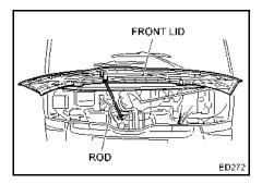
3. When opening the front lid, be sure to set the lever into the hole that is indicated with the mark located on the front lid.
