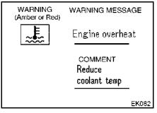
it is recommended to idle the engine until the ECT drops, then stop the engine and check the engine coolant level (ECL), and then inspect the cooling system for leaks.
