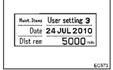
To change the display to the input screen of the periodic replacement intervals, push the mode select switch or the select switch for more than 1 second or turn the return switch for more than 1 second while the maintenance and inspection screen is displayed. A cursor will be displayed on the year position.
