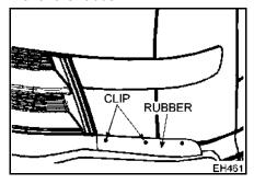
Remove the fixing clip from the lower cover, slide the lower cover downward and remove it.
