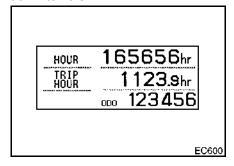
The hour meter continuously counts and displays up to 199999 hours.
