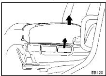
The rear of the driver's seat can be raised by pulling up the lever at the left side of the seat base.
