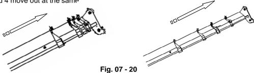
After the boom extends to required position, slowly tilt the pedal backward to neutral position;
