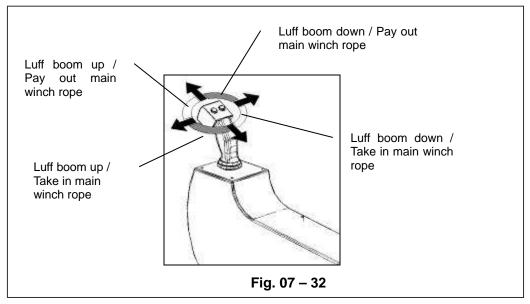
Move the right joystick between any two adjacent arrows to initiate required crane movements.
