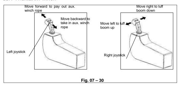
Move left and right joysticks at a time to initiate required crane movements.
