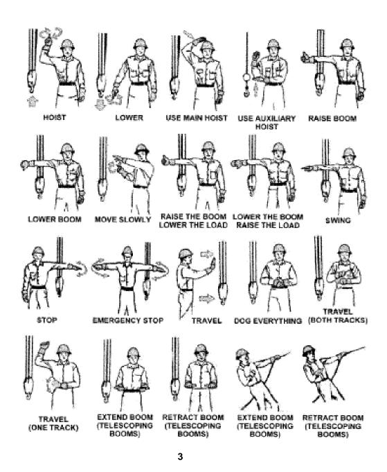
Figure 04 – 4 Hand Signals for Crane Operation
