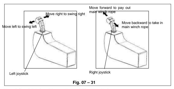
Move left and right joysticks at a time to initiate required crane movements.
