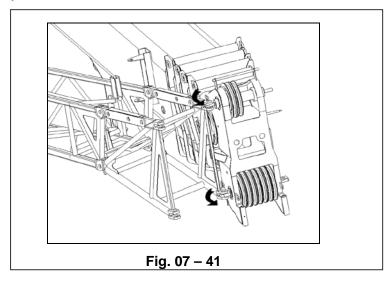
h) Connect at points D and E by inserting pin IV and guarding with load-spring pins;
