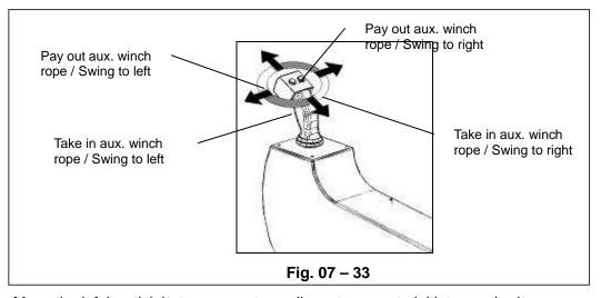
Move the left joystick between any two adjacent arrows to initiate required crane movements.
