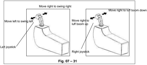
Move left and right joysticks at a time to initiate required crane movements.
