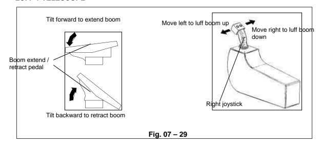
Move the right joystick and tilt the boom extend / retract pedal at a time to initiate required crane movements.
