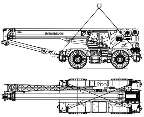
Figure 08 – 1 Crane Lift Points
