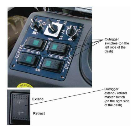
Figure 07 – 4 Outrigger Switches
