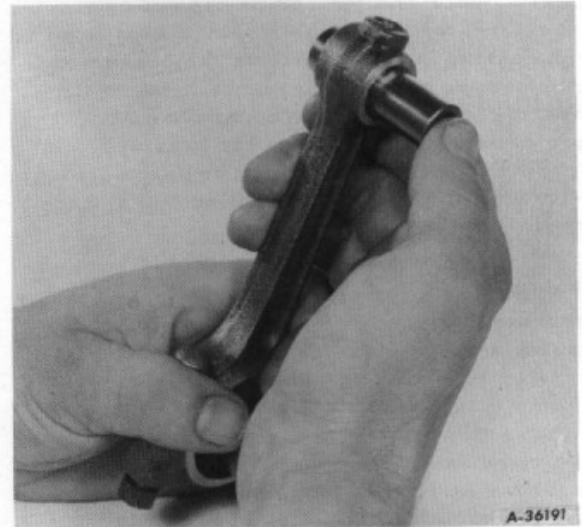
Illust. 8 -- Checking piston pin fit in connecting rod
