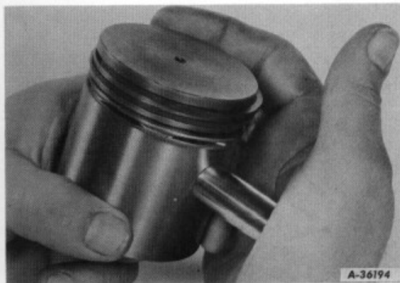
Illust. 18 -- Checking piston pin.
