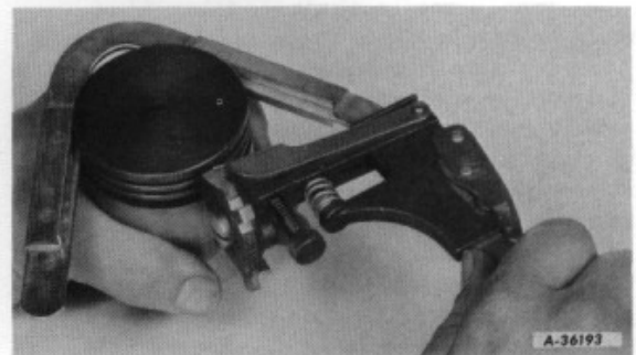
Illust. 16 -- Cleaning piston ring groove.
