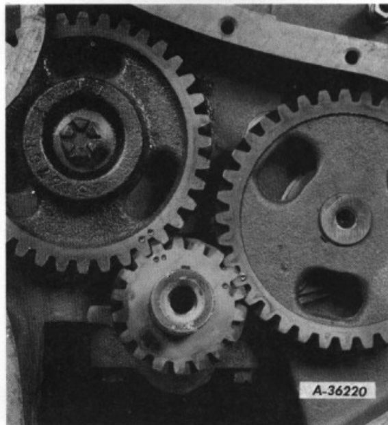
Illust. 43 -- Timing marks on camshaft, crankshaft and idler gears.
