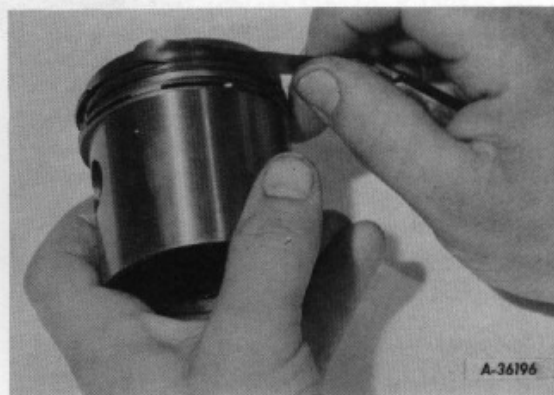
Illust. 20 -- Checking piston ring clearance in groove.
