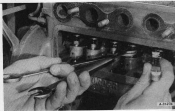
Illust. 45 -- Adjusting valve tappets.
