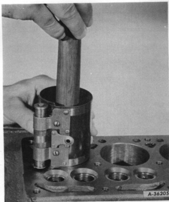
Illust. 44 -- Using piston ring compressor to install pistons.
