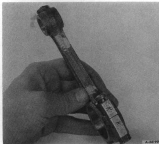
Illust. 6 -- Connecting rod and bearing cap markings.
