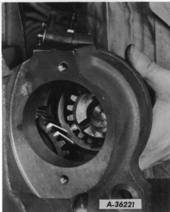
Illust. 50 -- Installing governor and ignition drive gear. Note chalk marked gear teeth in proper position.
