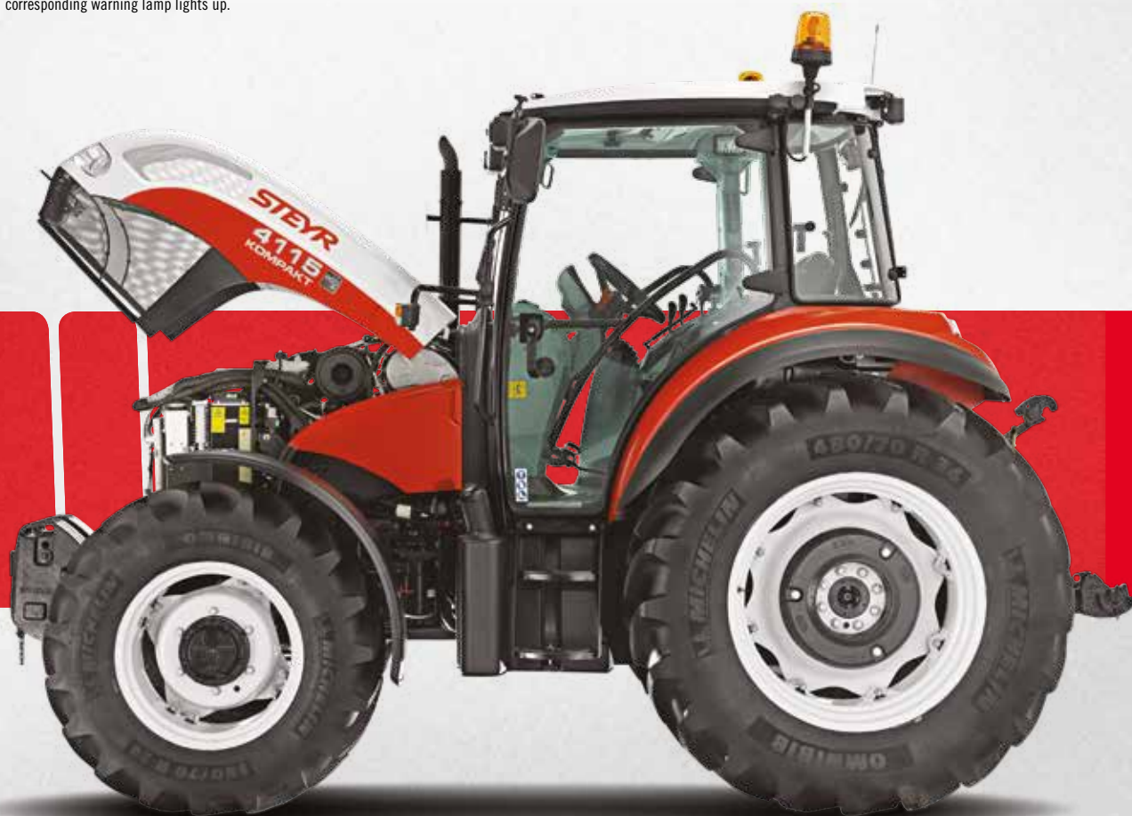
One-section bonnet on gas struts can be raised, even when a front-mounted implement is attached.
