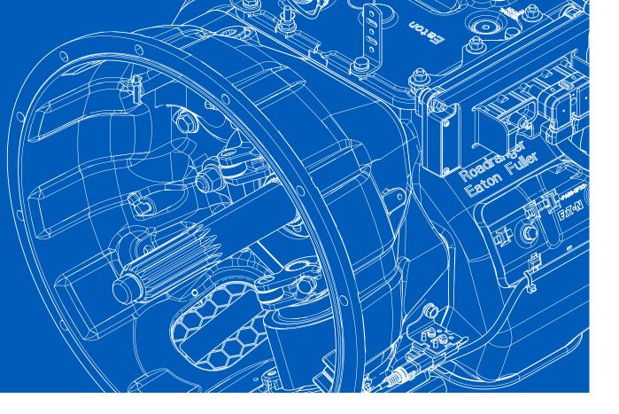
The strategic use of aluminum components, combined with a durable, sculpted-iron case and the elimination of the oil cooler and lines, shaves off up to 82 pounds from the system.
