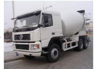
DAYUN Cement mixer truck is dayun brand truck chassis, it can build 9, 12, 14 cubic meters mixer tank. EATON, Bonfiglioli Riduttori, ARK, ZF mixer parts including Hydraulic motor, reducer, oil pump.
