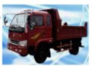
Length x width x height5965× 2200× 2450 mmWheelbase3400mmFront / Rear wheel track1770/1640 mmFront /Rear suspension1185/1380 mm
