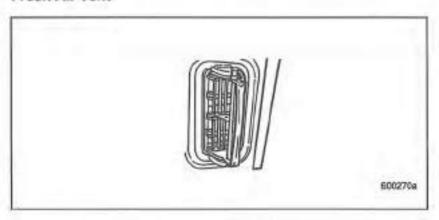
An air vent is provided to circulate outside air to the cab interior. Move the vent lever forward or rearward to open the vent. Move the lever to the center to close the vent.
