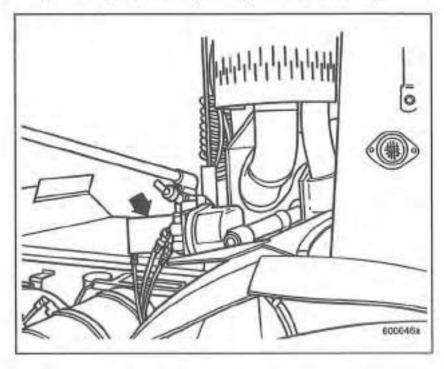
To raise to the <u>service</u> position, pump the cab up to the SERVICE HEIGHT position.
