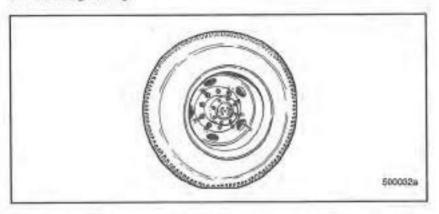
Look for cracks around the hand hole, stud hole and wheel. Look for broken studs, wheel damage or improperly seated lock rings.
