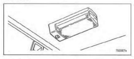
The dome lights are located in the cab headliner. With the switch in the left position, the dome light will come on when the cab door is opened and go off when it is closed. Push the switch to the right to turn on the dome light when the doors are closed.
