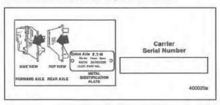
The MERITOR rear axle identification tag is located on the left or right rear of the rear axle housing, next to the carrier.
