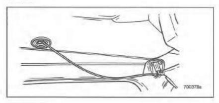
The air horn(s), if equipped, is activated by pulling down on the cord that is located above the left-side window.
