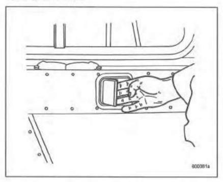
The inside door handles are flush-mounted, with paddle-type design. To open the door, grasp the handle and pull out while exerting some force on the door.
