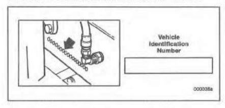
The VIN plate is located on the driver side, mounted on the seat riser.
