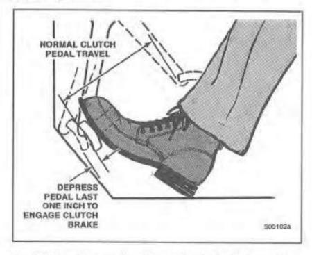
With the vehicle standing still, apply the clutch brake by pushing the clutch pedal all the way to the floor; the clutch brake is applied when the clutch pedal is <u>fully depressed</u> (the last one inch of travel past normal pedal travel).
