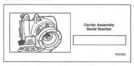
The Eaton Fuller rear axle serial number is located on the rear of the axle housing toward the carrier.
