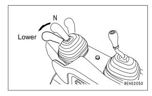
6. Lock blade control lever (5) and ripper control lever (6) with safety lever (7).
