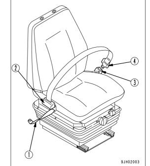
Check that the bolts of the clamp securing the belt to the chassis are not loose. Tighten them if they are loose. The tightening torque for the mounting bolt is  $24.5 \pm 4.9 \, \text{N} \cdot \text{m}$  ( $2.5 \pm 0.5 \, \text{kgf} \cdot \text{m}$ ).
