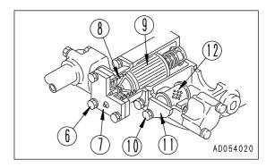
Replace the power train filter element.
