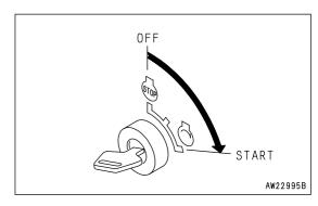
3. When the engine starts, release the key in starting switch (2). The key will return automatically to the ON position.
