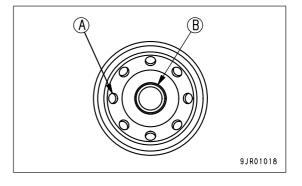
4. When installing, tighten until the packing surface contacts the seal surface of the filter holder, then tighten it up 1/2 to 3/4 of a turn.
