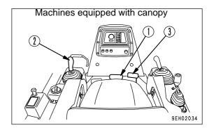
Depress brake pedal (1) to stop the machine.
