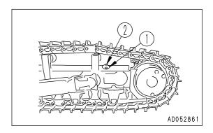
2. Add grease through the grease fitting marked by the arrow.
