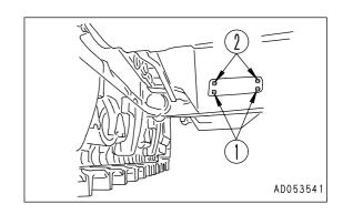
Apply grease to the grease fittings (2 places) shown by arrows.
