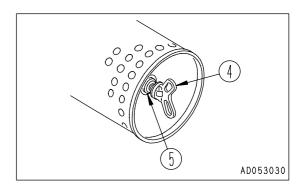
Direct dry compressed air (less then 700 kPa (7 kg/cm², 100 psi)) to the element from inside along its folds, then direct it from outside along its folds and again from inside.
