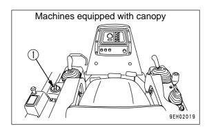
Turn fuel control dial (1) to the center position between LOW IDLING (MIN) and HIGH IDLING (MAX) and run the engine at medium speed for about 5 minutes with no load.
