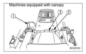
Depress decelerator pedal (2) and reduce the engine speed.
