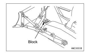
2. Loosen set bolt (1) of the brace, insert a suitable bar into hole (2) of the brace, and turn it.
