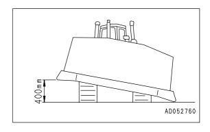
1. Raise the blade 300 - 400 mm above the ground, then put blocks under the frame so that the blade does not come down.
