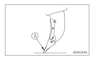
Choosing a suitable ripper point to match the type of rock is one of the most important elements in using the ripper effectively.
