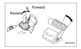
3. After depressing decelerator pedal (2), move joystick (1) to the desired position.
