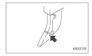
If the wear exceeds the wear limit in the table below, replace the worn parts.
