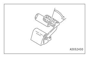
2. Return joystick (1) to the neutral position, reduce the speed, then depress brake pedal (3) and stop the machine.
