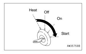
5. When the engine starts, release the key in starting switch (2). The key will return automatically to the ON position.
