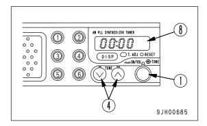
When the sound suddenly disappears and appears again, the button is programmed, and the preset number is shown in display area (8).
