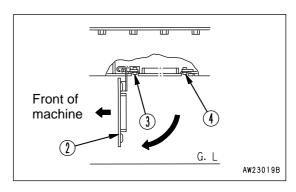
6. Install undercover (2), then close engine side cover (1) at the left side of the machine.
