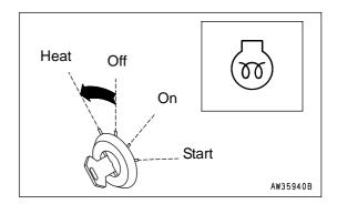
While preheating is being carried out, the preheating pilot lamp (3) lights up to show that preheating is being carried out. After it lights up for 36 seconds, it flashes for 16 seconds and goes out. When it goes out, complete the preheating immediately.
