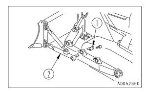
3. Insert arm (2) into the desired position on the bracket on top of the frame (3 places on each side), and insert pin (1).
