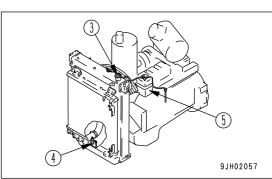
12. Replace the corrosion resistor, and turn valve (1) to the OPEN stopper position.
