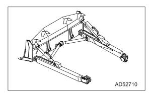
2. If a greater tilt amount is needed, use adjustment bar (2) installed to left brace (1) to rotate brace (1) and change the brace length.
