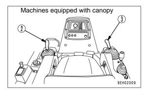
Check that parking lever (1) is locked. If this lever is not at the LOCK position, the engine will not start.
