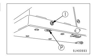
1. Lower the blade to the ground, stop the engine and wait for about 5 minutes before checking oil level. If the oil level is between H and L in sight gauge (G), it is normal.
