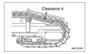
Check the clearance between the idler guide plate and the track frame. If clearance (B) increases, idler may develop side motion and tracks may come off. (For inspection and adjustment procedures, refer to "ADJUST IDLER CLEAR-ANCE (PAGE 4-35)".)
