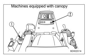
1. Turn fuel control dial (1) to the low idling position and run the engine at low idling speed for about 5 minutes to allow it to gradually cool down.
