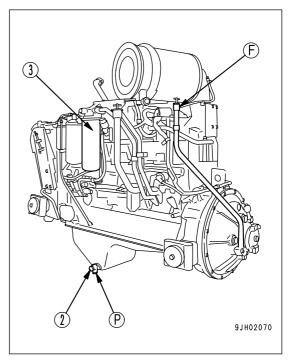
Clean the filter holder, fill the new filter cartridge with engine oil, coat the packing surface and thread with engine oil (or coat it thinly with grease), then install the filter cartridge.
