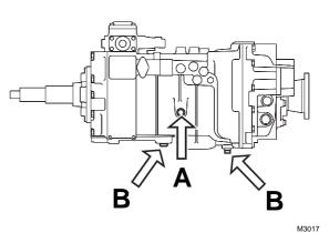
4. Remove the drain plugs (B and C) and the level check/filler plug (A) and drain the oil.
