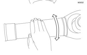
3. There must be no clearly noticeable play on universal joints and centre bearing.
