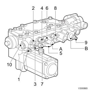
Rear view of integrated air distribution block
