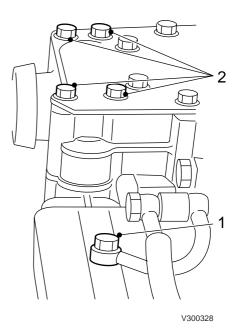
Pneumatically assisted gearbox control (Servoshift)
