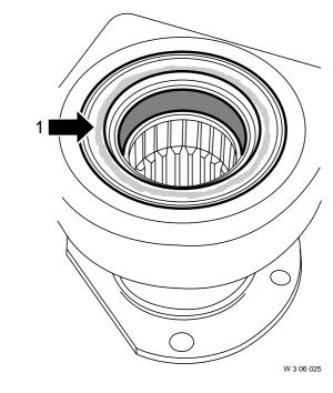
2. Press the bearing along the other side into the bush. Then the other sealing ring can be pressed into the bush. Apply grease to the sealing rings (1).
