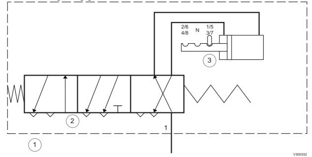
When the cylinder is in the 2<sup>nd</sup>/6<sup>th</sup> or 4<sup>th</sup>/8<sup>th</sup> position and the gear lever is again released, the selector valve will again spring back to the middle position while the cylinder remains in the switched position due to the double-retaining arrangement.
