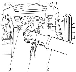
3. Fit the torque rod to the control rod and tighten the ball joint lock nut (4) to the specified tightening torque.
