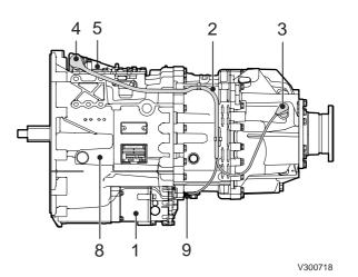
With AS Tronic gearboxes, the clutch is operated fully automatically by the electropneumatic clutch unit (1), which, in its turn, is controlled by the electronics inside the gearbox modulator (5). The wiring harness (2) connects the clutch unit to the modulator (5). The wiring harness connects the clutch unit (9) to the gearbox modulator (5) via a connector (4).
