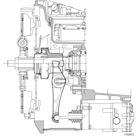
A diaphragm spring requires a self-centring thrust bearing.
