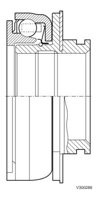
The thrust bearing with plastic coating can be recognised by the spline-shaped inner diameter.
