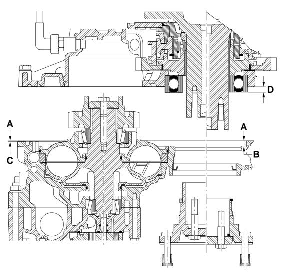
1. Measure and note down distance "A - C" from sealing surface A with gasket to contact surface C.
