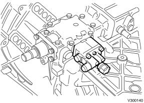
Gate protection valve At the left-hand or right-hand side of the gearbox (depending on the vehicle type). 2.
