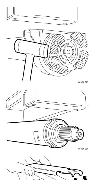
7. Remove the lock plate from the mounting bracket.
