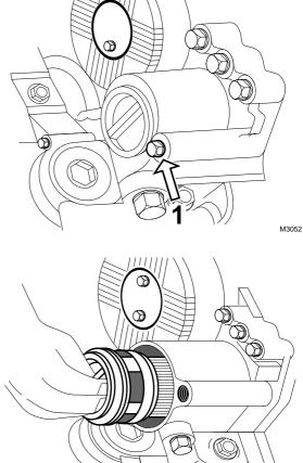
2. Pull the filter cover with the filter from the filter housing.
