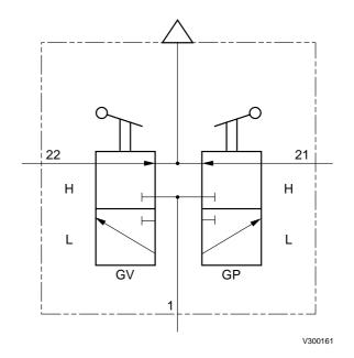
Pneumatic section of gearbox
