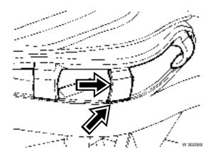
Then remove the Seeger ring that has become visible from the bearing cover. It is 3. now possible to remove the entire gear lever from the bearing cover.
