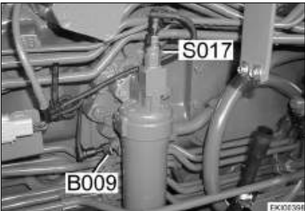
S017 = Switch, filter clogging Behind right rear wheel on pressure filter
