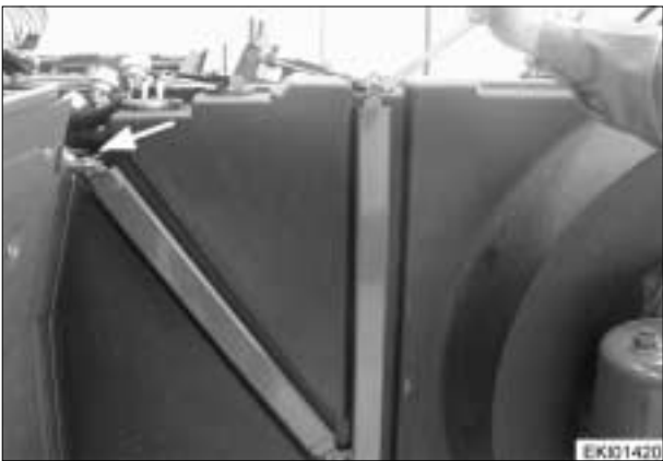
Fit clamp, brace and bracket (arrowed).
