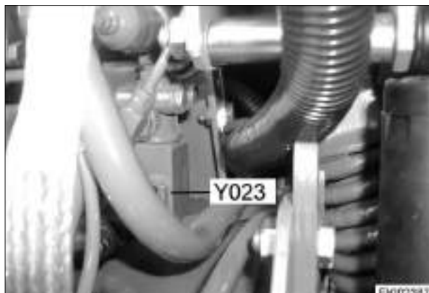
Y023 - 3-way directional control valve (pilot valve)
