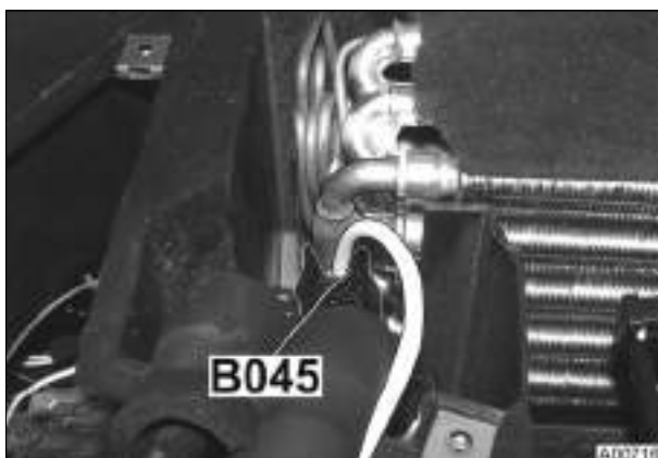
B045 = Sensor, air-conditioning 2 Top right between A- and B-pillars at air-conditioning expansion valve
