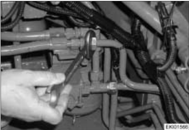
Fit hydraulic lines to front power lift.
