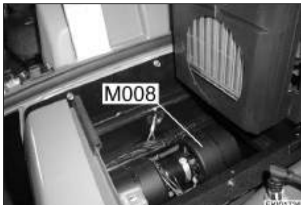
M008 = Motor, heater fan In front of cab
