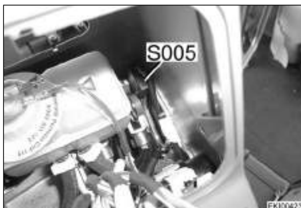
S005 = Solenoid switch, right brake At top on brake pedals
