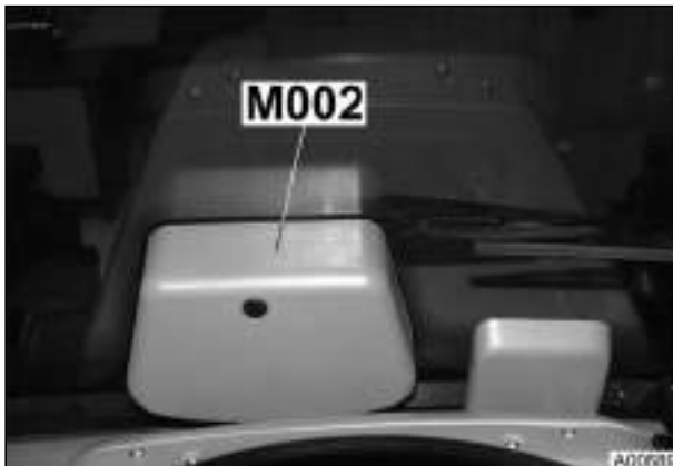
M002 = Wiper motor, front In windscreen
