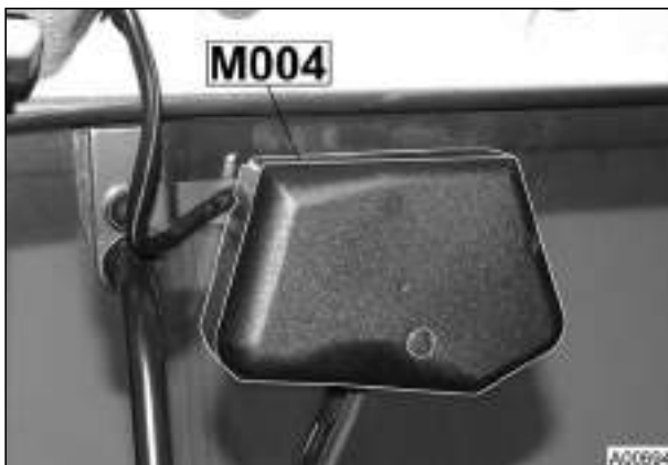
M004 = Wiper motor, rear In rear window
