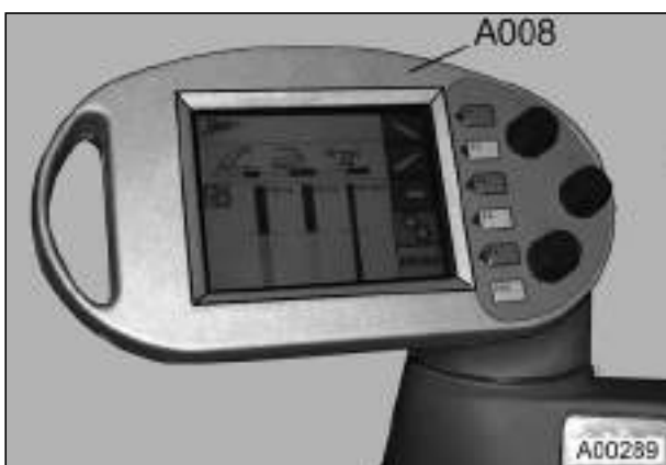
A008 = Vario terminal On right in cab on control console
