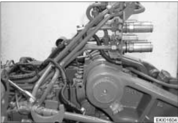
Fit hydraulic lines for EPC-DA switchover.
