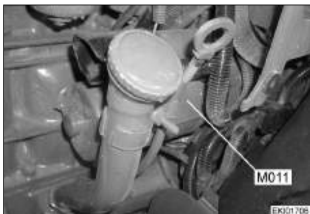
M011 = Starter motor, 24V Left rear on engine
