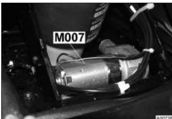
M007 = Motor, seat adjustment Under seat bracket
