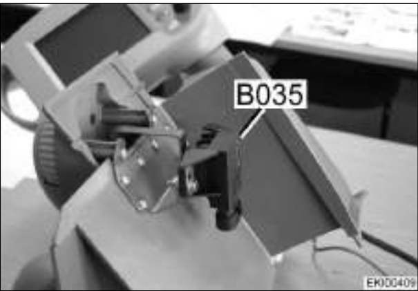
B035 = Sensor, hand throttle In control console
