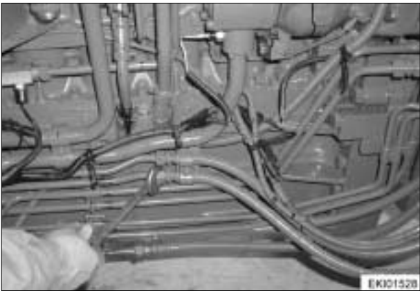
Fit hydraulic lines to steering cylinder.
