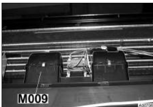
M009 = Motor, fan Top front in roof
