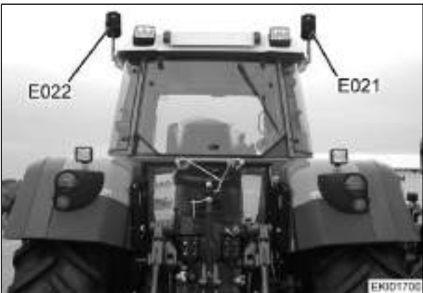
E021 = Rotating beacon right E022 = Rotating beacon left Tractor seen from rear
