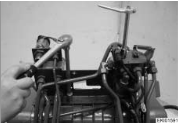
Fit bracket for hydraulic couplings.
