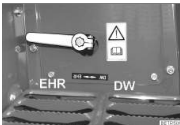
Fig. 8 Fav 700 rear power lift EPC/DA switchover AV3/AV4 with solenoid switch S048 (behind cover panel)
