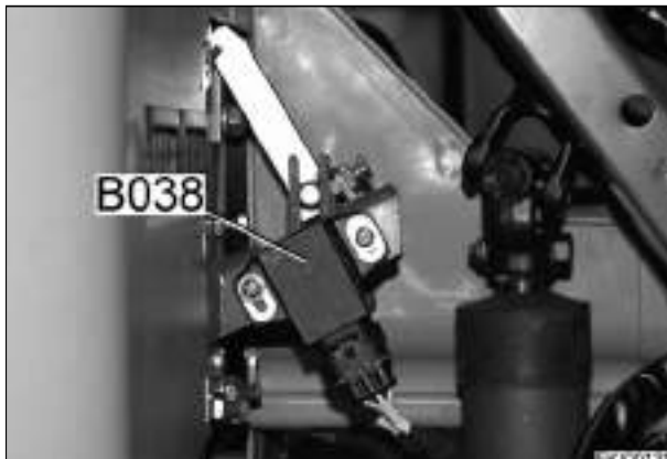
B038 = Sensor, accelerator Cab, under steering column
