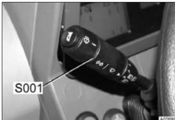
S001 = Switch, control stalk On left of steering wheel
