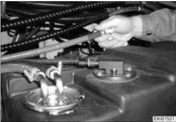
Fit tank venting tube.
