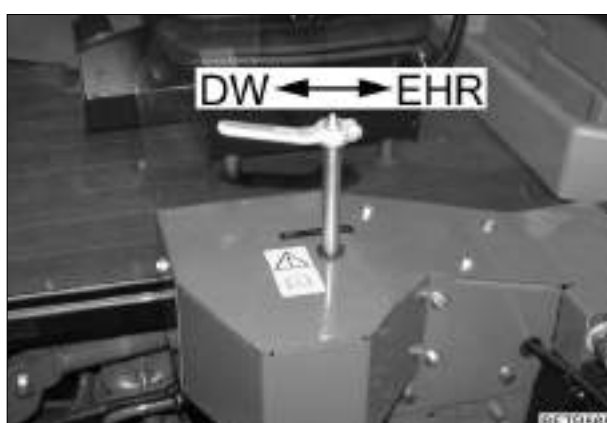
Fig. 9 Fav 900 rear power lift EPC/DA switchover AV3/AV4 with solenoid switch S048 (behind cover panel)
