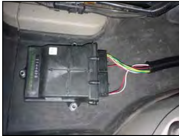
FIGURE 6. Node harness Connected to the Node
