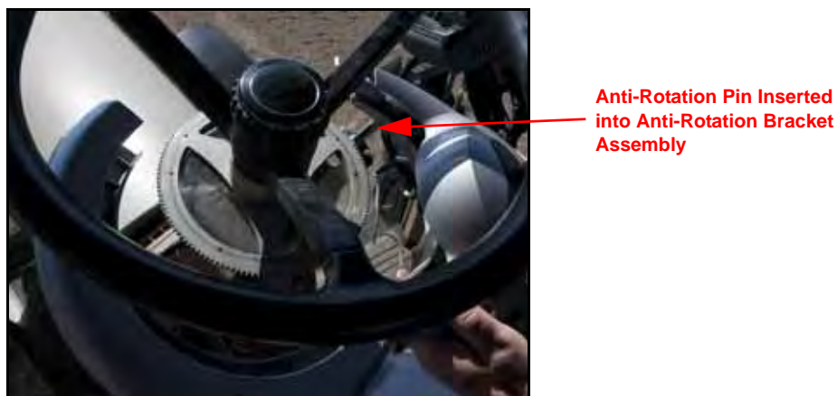
FIGURE 16. Anti-Rotation Pin Installed in Bracket Assembly
