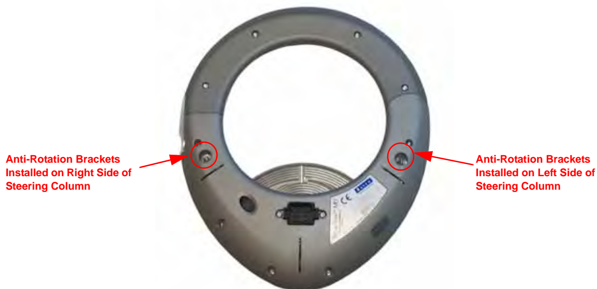
FIGURE 15. Anti-Rotation Pin Installation Locations
