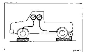
PINSTALL LSPV GAUGE (SST) AND BLEED AIR
