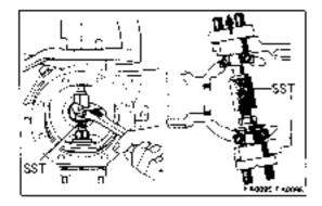
(c) Using SST, push out the knuckle arm and shims from the steering knuckle.
