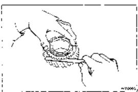
(b) Measure the clearance between the synchronizer ring back and the gear spline end.
