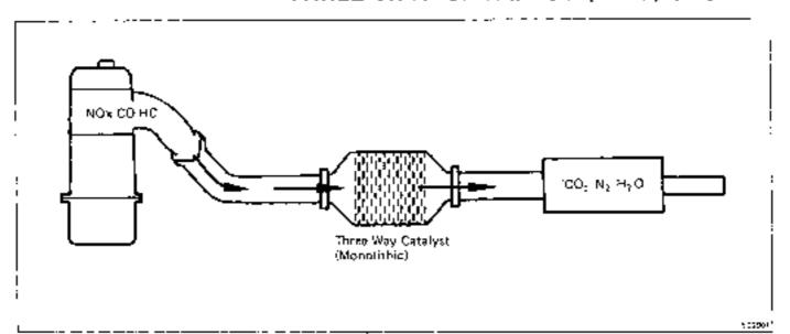
To reduce HC, CO and NCx emissions, they are oxidized, reduced and converted to nitrogen (Nz) carbon dioxide  $\langle \text{CO} \rangle$  and water Im/OI by the catalyst.
