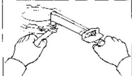
[8] Install a new pressure place with the special pressure plate bolts and nuts. Torque the nuts.
