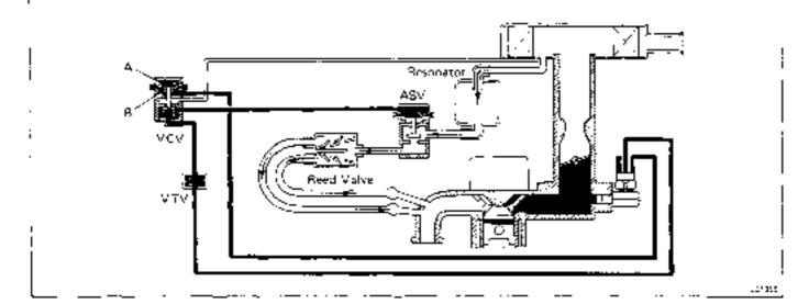
To reduce HC and CO emissions, this system draws in air into exhaust corts to accelerate oxidation, using vacuum generated by the exhaust polsation in the exhaust mainfold
