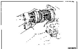
Idi Disengage the gear double meshing.
