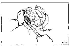
ld). Using a torque meter, measure the preload.
