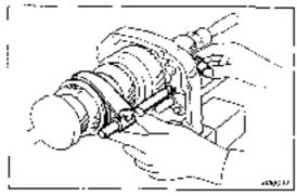
(g) Remove the shift fork and shaft No. 2.
