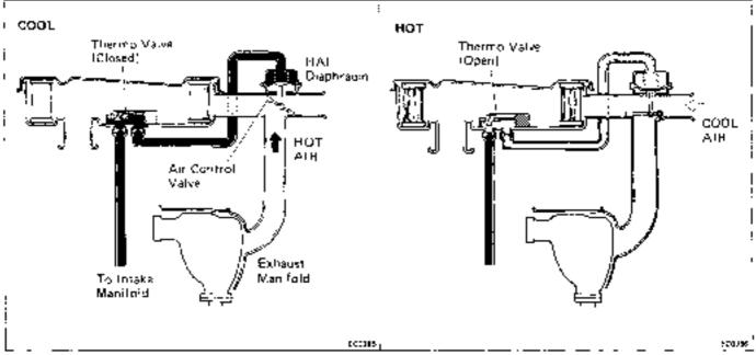
This system leads a horiair supply to the carouretor in cold weather to improve driveability and to prevent the carburetor from using in extremely cold weather.
