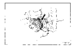
(d) Install the 5th gear assembly with the synchronizer ring slots augued with the shifting keys.
