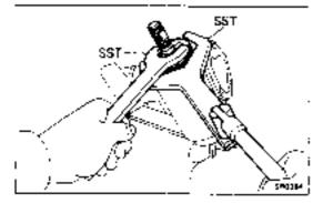
(c) Hold the adjusting screw in position with SST and tighten the lock nut with SST.
