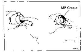
(b) Apply MP grease to release bearing.
