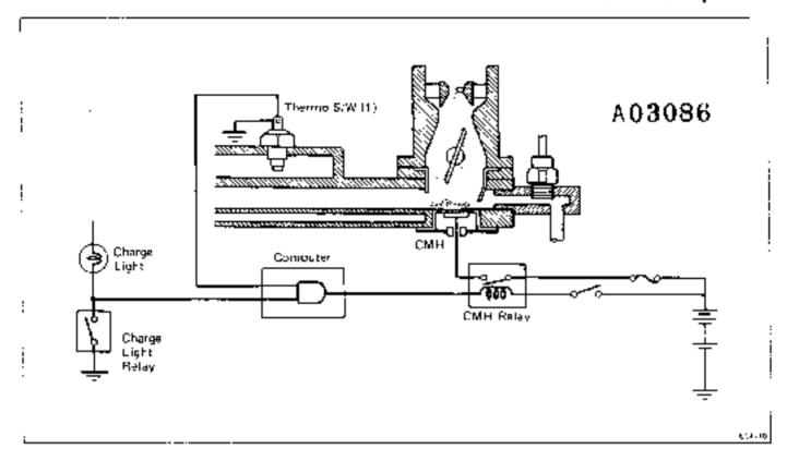
To reduce cold engine emission and improve drivability, the intake manifold risor is heated during cold engine operation to accelerate vapor-zerion of the liquid fuel.
