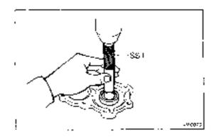
(b) Using SST, press in the oil seal.
