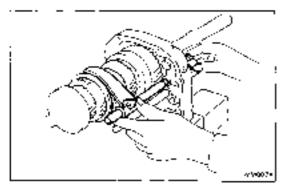
(3) Install fork shaft No. 2 to the shift fork through the intermediate plate
