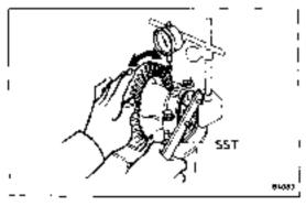
(h) Using a dial indicator, adjust the ring gear backlash until it is within specification.
