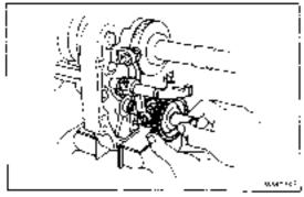
(b) Install the reverse idler gear and shaft.
