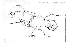
The most frequent cause of problems is simply a bad contact in wiring connectors. So always make sure that connections are secure.
