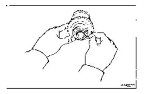
18) Select a snap ring that will allow minimum axial play and install it on the shaft
