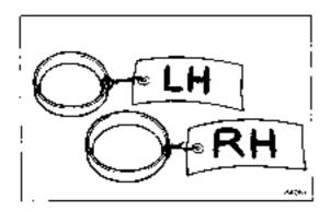
NOTE: Tag the disassembled parts to show the location for reassembly.
