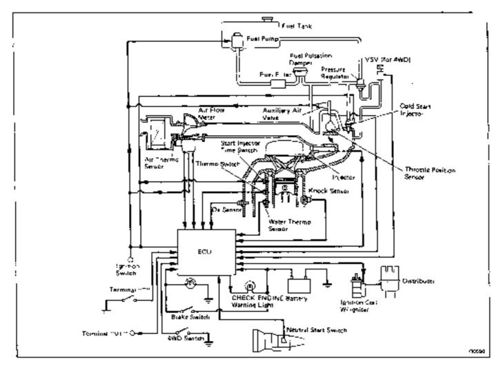
The EFI used on Toyotas has three basic systems.
