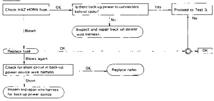
NOTE: Back up power refers to the storage voltage run preset tuning. This is applied even when the ignition switch is OFF.
