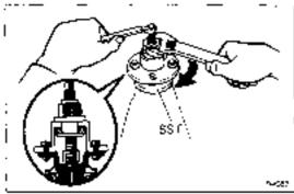
(c) Adjust the drive pinion preload by tightening the companion flange nut.
