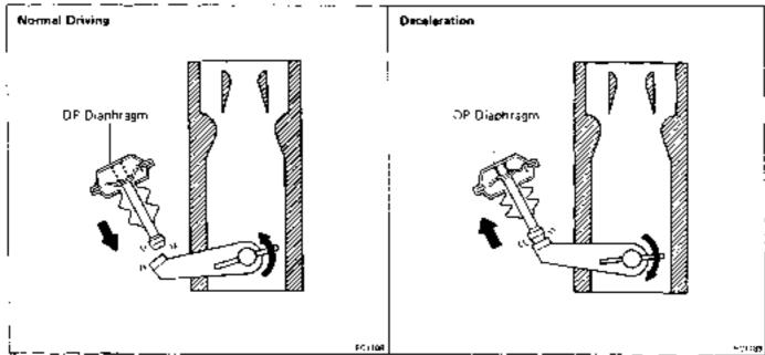
To reduce HC and CG emissions, when decelerating the dash por opens the rhintitle valve slightly more than arrible this causes the air-fuel mixture to burn completely.
