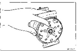
(c) Install the rear suction valve over the pins on the rear cylinder.
