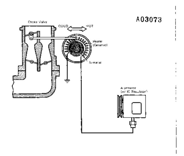
This system temporarily supplies a nich mixture to the engine by closing the choke valve when the engine is cold Current from Choke Valve **IG 5/W** Burmeral . Terminal Lito Heater , CFF Not Howing Excanded CLOSED C. DSEU E-panded Not rubning QM. Heated up and contracted OPEN Hunding Flowing. emarks 10n alternators with an IC requistor, sight voltage will becomwhen the ignition switch is turned ON, bur not sufficient current to warm up the heater
