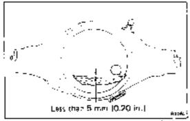
INSTALL DRAIN PLUG AND FILL DIFFERENTIAL WITH GEAR OIL
