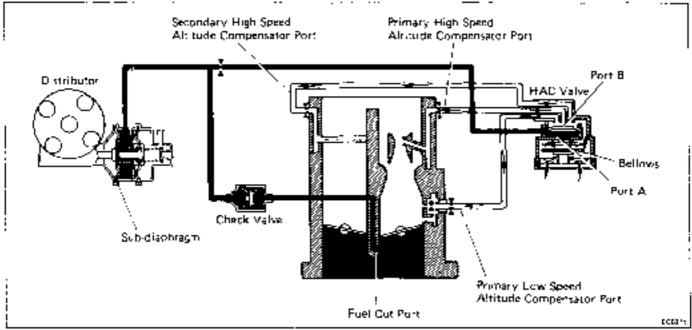
As a titude intreases, the air-fuel mixture becomes richer. This system insures proper air-fuel mixture by supplying additional air to the primary low and high speed circuits and secondary high speed circuit of the carouretor, and advances the ignition timing to improve drive above at high actuals labove 3,198 m (3,990 ft).
