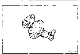
If the speed is not as specified, unlock the lock nut, and adjust the setting speed by turning the dash pot diaphragm.
