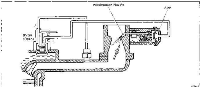
The Carburetor air-line mixture is very loan. When accelerating with a cold engine, the main acceleration pump capacity is insufficient to provide good acceleration. The AAP system compensates for this by forcing more find into the acceleration notice to octain bester cold engine performance.
