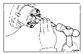
(d) Using a tapered punch, tap the slits of the cone washers and remove them.
