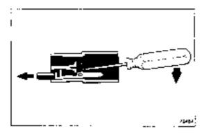
(b) Pry up the locking fug with the screwdriver and pull the terminal out from the rear.
