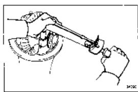
(i) Torque the bearing cap bolts.
