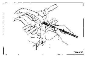
Ib) Using a magnetic finger, remove the three springs and balls.
