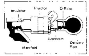
Install the injector to the delivery pipe and intake manifold as shown in the figure.
