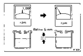
3. CHECK THAT FLUID IN RESERVOIR IS NOT FOAMY OR CLOUDY AND DOES NOT RISE OVER MAXIMUM WHEN ENGINE IS STOPPED
