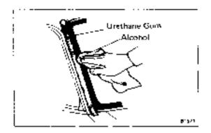
(b) Clean the cutting surface of the urethane gum with a piece of cloth saturated in solvent falcohol).
