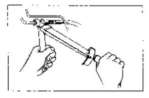
(c) Then tighten the nut to the specified rorque.
