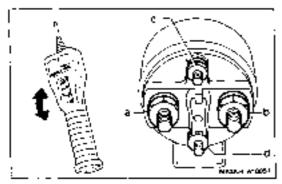
Check operation of sub-magnet switch A and B, with the remote control switch in the NEUTRAL position.
