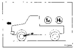
(c) For transfer, shift to H2 and proceed slowly. During this, one person should check under the vehicle to see that the propeller shaft is turning. If turning this means that the automatic locking hub incoked.
