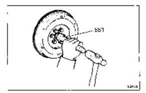
(b) Using SST, install the pilot bearing SST 09304-30012
