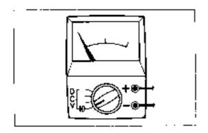
4 Use a volt/ohometer with a high impedance ITO kB/V minimum) for troubleshooting an electrical circuit.
