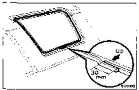
(c) Install the seal to the cover top body.
