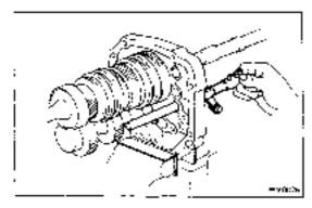
(i) Remove fork shaft No. 3 with reverse shift arm.
