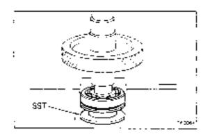
lcl Using SST, press in a new bearing, SST 09316-60010
