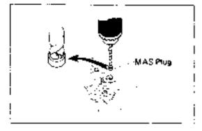
(e) Use a 7.5mmφ (0.295 in.φ) drill to force the plug off.
