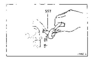
(c) Using SST, tighten the four plugs. SST 09312-30021
