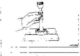
(b) Using a press, remove the bearing.
