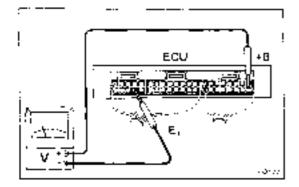
NOTE: 1 Perform all voltage measurements with the connectors connected.
