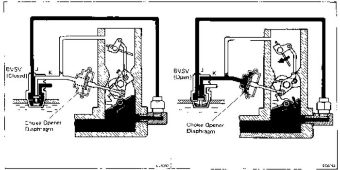
After warm-up, this system forcibly holds the choke valve open to prevent an over-rich mixture and release the fast, did cam to the 415 step to lower the engine rpm.
