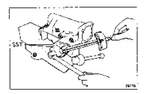
(c) Using SST, tighten the lock nut while holding the bearing cap with SST.
