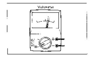
6. CHECK THAT NEEDLE OF VOLTMETER FLUCTUATES 8 TIMES OR MORE IN 10 SECONDS
