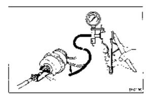
(c) Disconnect terminal 2 or 3 and check that the control cable returns to its original position and the vacuum returns to 0 mmHg (0 in Hg, 0 kPa).
