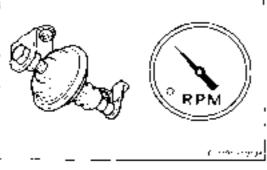
(b) Release the throttle valve gradually, and check the dash pot setting speed when the throttle lever touches the dash pot end.
