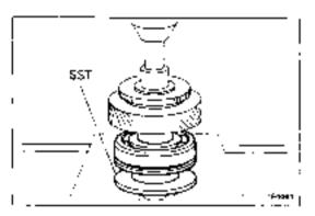
(c) Using SST, press in a new bearing. SST 09316-60010
