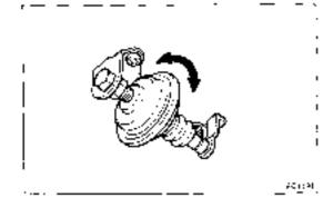
If the speed is not as specified, unlock the lock out, and adjust the sotting speed by turnning the DP diaphragm.
