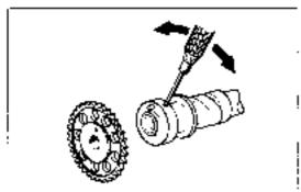
Place the chain sprocket over the camshaft dowel. NOTE: If the chain does not seem long enough, turn the camshaft back and forth while pulling up on the chain and sprocket.
