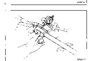
(b) Temporarily assemble the joint and measure the joint. radial play with a dial indicator.
