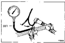
(g) Install a gasket, SST, another gasket and union bolt to the delivery pipe as shown in the figure.
