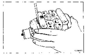
(b) Using a hammer and punch, remove the front housing by tapping on the protrusion.
