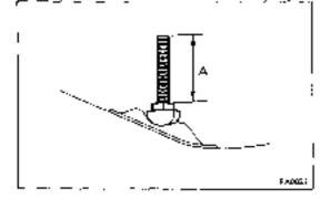
(f) Tighten the adjusting nut so that the bolt protrusion is equal to that before removal.
