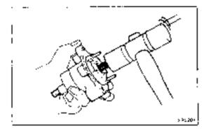
(d) Using a plastic hammer, lightly tap the rotor shaft out of the front housing.
