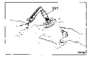
(b) Using a torque wrench and SST, measure the bearing preload in both directions. Turn the adjusting screw until the preload is correct.
