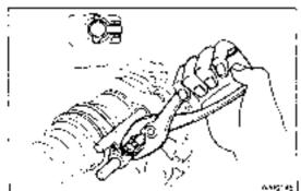
Using pliers, stake the bolts with lock washers.
