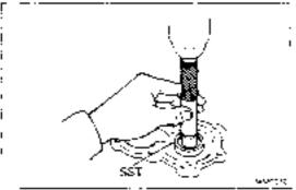
(b) Using SST, press in the oil seaf.
