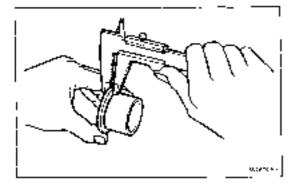
Using calipers, measure the inner race flange thickness.
