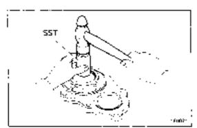
(b) Using SST, drive in a new oil seal.
