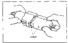
(b) Fully insert the connector and insure that it is locked.
