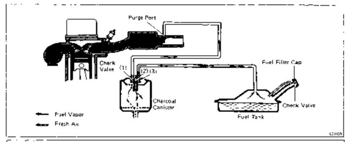
To reduce HC emission, evaporated fuel from the fuel tank is routed through the chargeal canister to the throttle body for combustion in the cylinders
