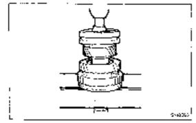
(d) Using a press, install the 2nd gear and hub sleeve No.1.
