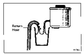
REMOVE FLUID RETURN HOSE FROM RESERVOIR TANK AND DRAIN FLUID INTO CONTAINER
