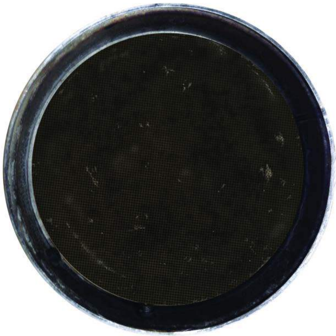
Figure 47 Diesel Particulate Filter (DPF) Inlet - Dirty, but Reusable.
