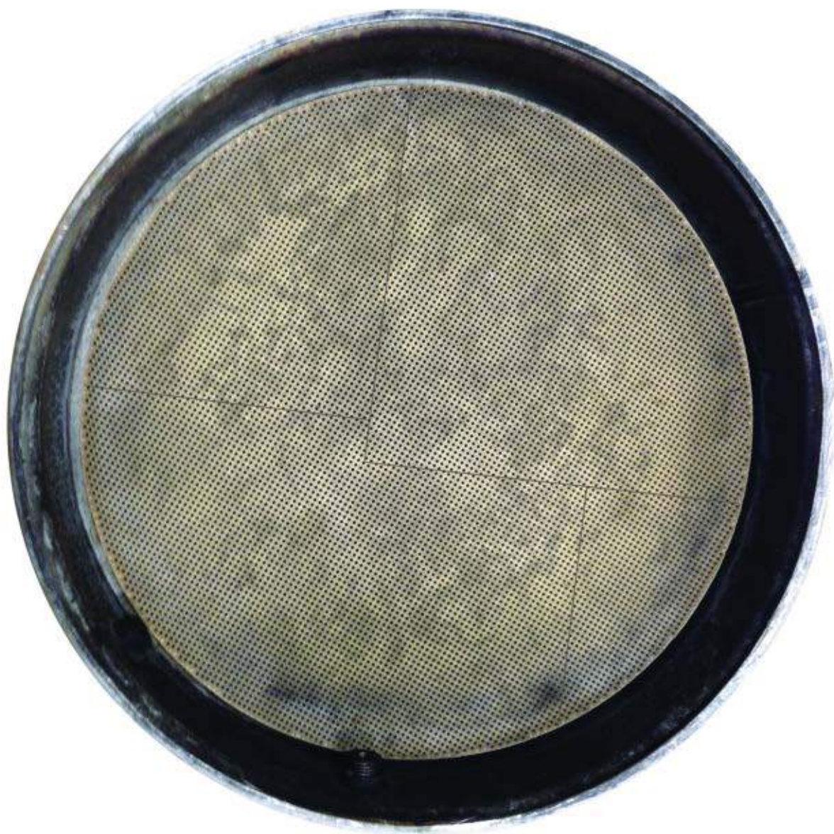
Figure 50 Diesel Particulate Filter (DPF) - Cracked, but Reusable.
