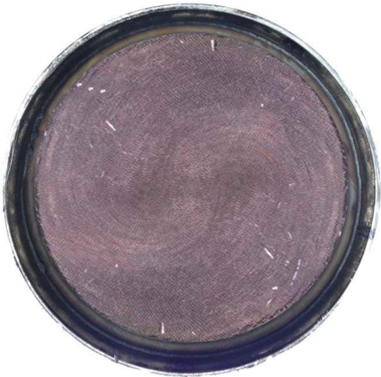
Figure 54 Diesel Oxidation Catalyst (DOC) Outlet - Dirty, but Reusable.
