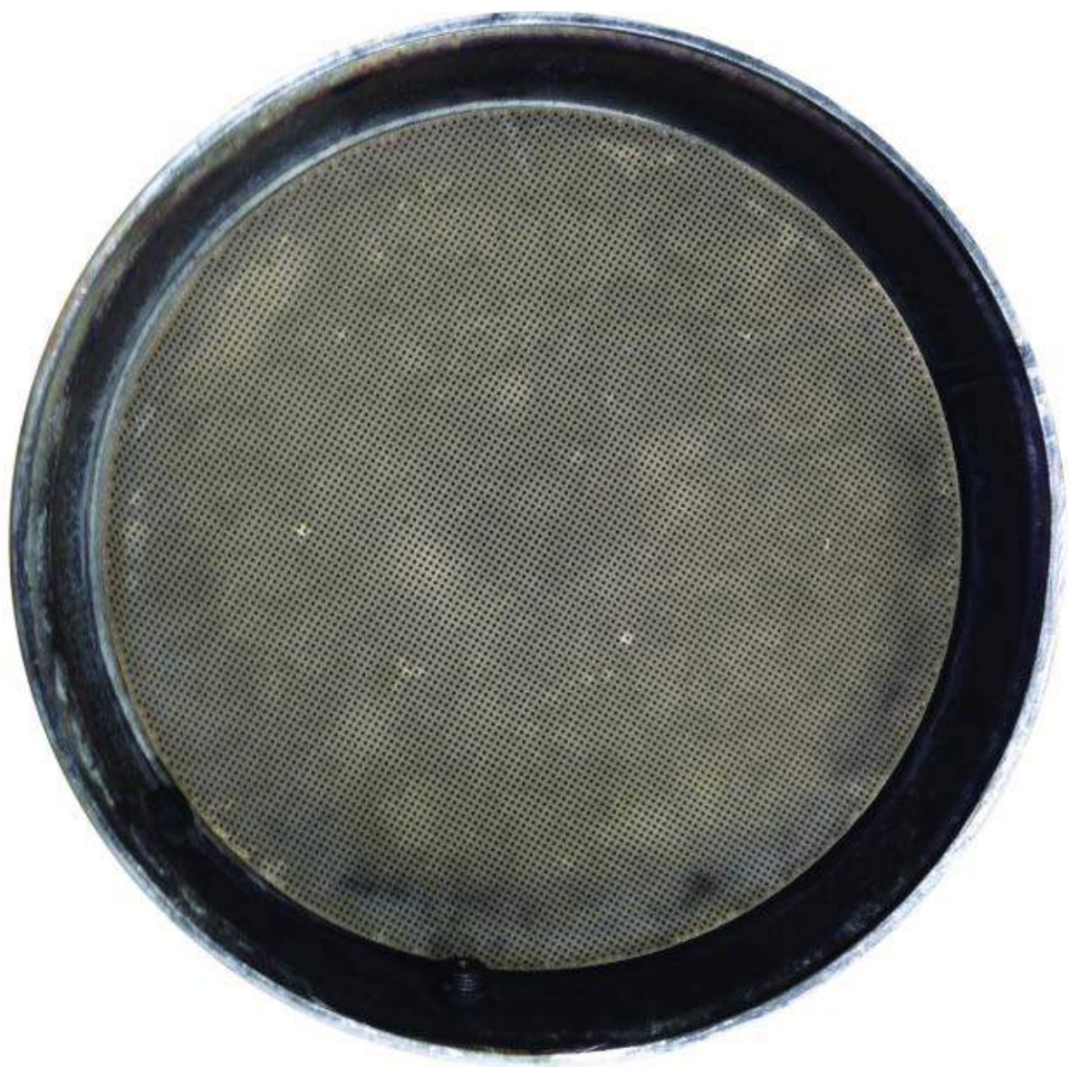
Figure 46 Diesel Particulate Filter (DPF) Inlet - Clean.
