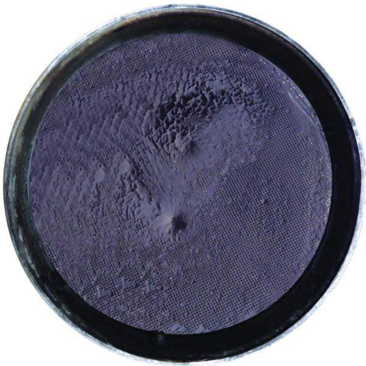
Figure 48 Diesel Particulate Filter (DPF) Inlet - Face Plugged.
