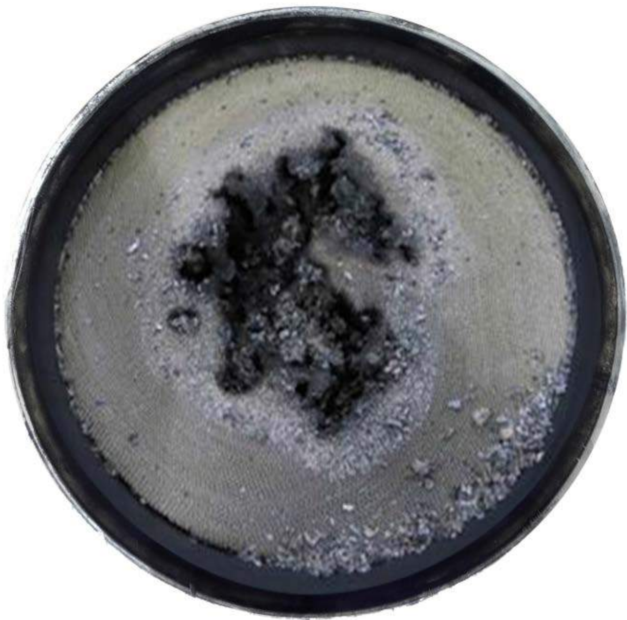
Figure 56 Diesel Oxidation Catalyst (DOC) - Melted.
