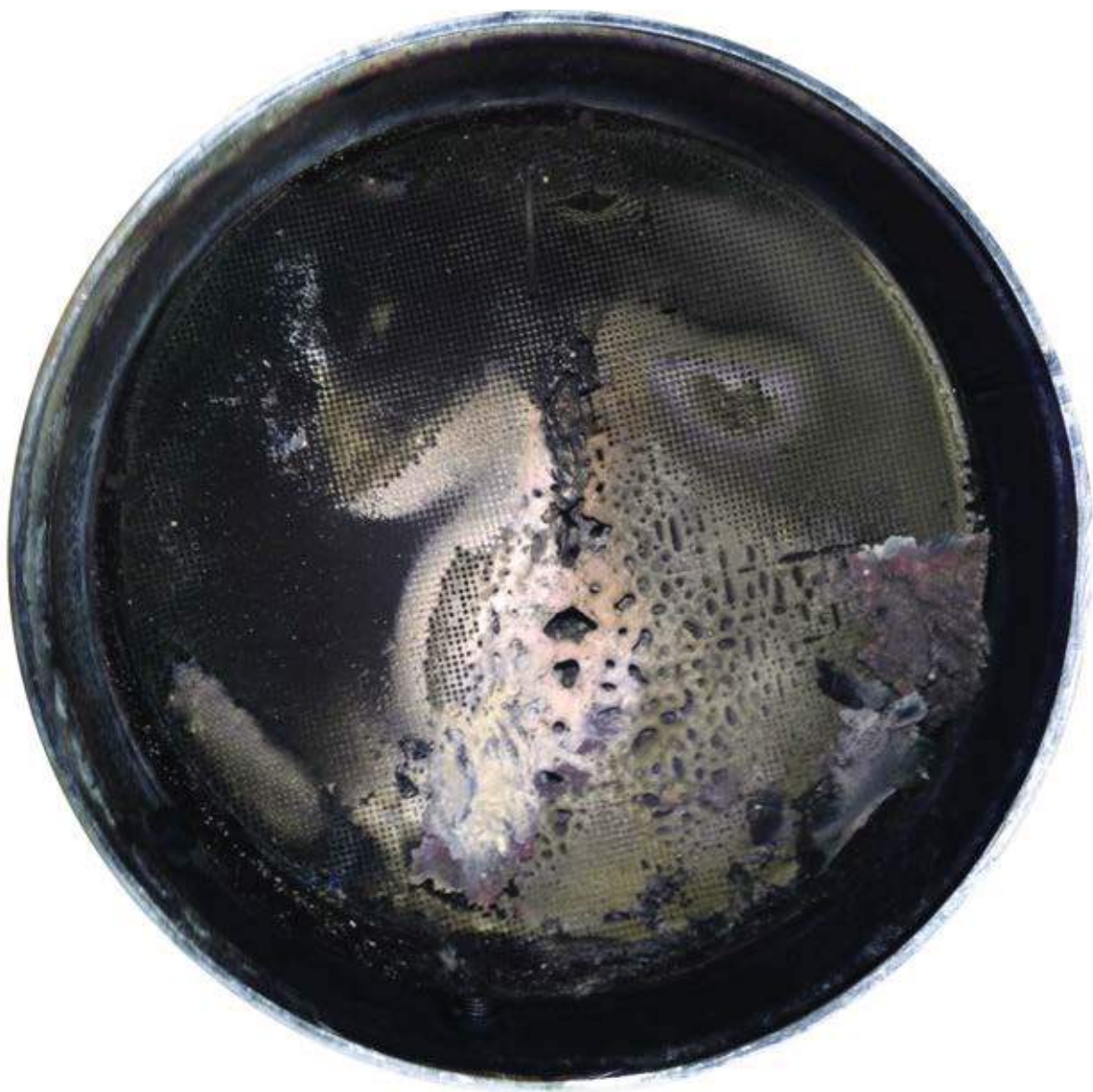
Figure 49 Diesel Particulate Filter (DPF) - Melted.
