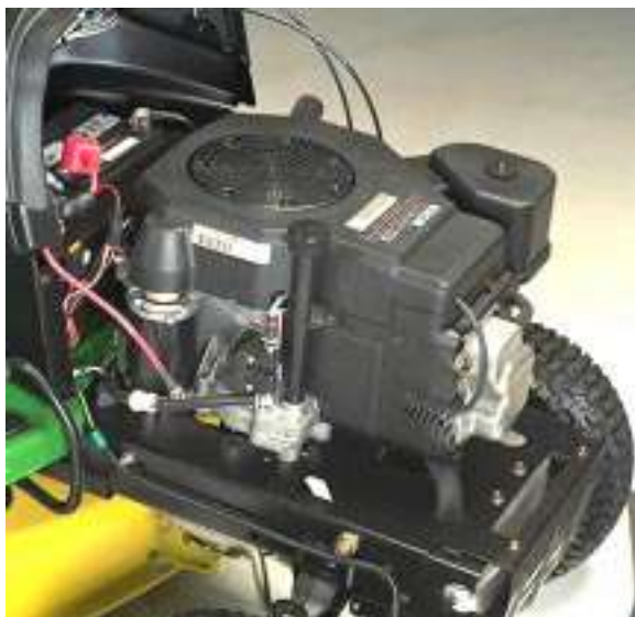
L110 17.5 horsepower Kohler engine shown
